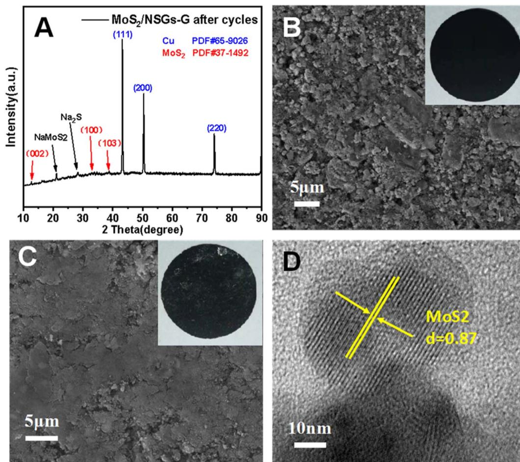
Fig. 6 XRD pattern of the MoS<sub>2</sub>/NSGs-G after 250 cycles (A), SEM images of the MoS<sub>2</sub>/NSGs-G electrode before 250 cycles (B), after 250 cycles (C), HRTEM image of the MoS<sub>2</sub>/NSGs-G after 250 cycles (D). Inset: corresponding digital photo of the MoS<sub>2</sub>/NSGs-G electrode before and after 250 cycles in SIBs.
