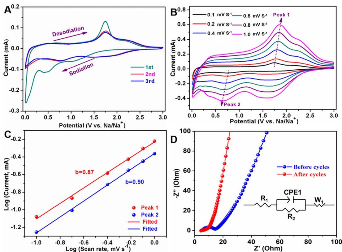
Fig. 4 Typical CV curves at a sweep rate of 0.1 mV s<sup>-1</sup> for the first three cycles (A), CV curves at different scan rates (B),  $\log(i)$  versus  $\log(v)$  plots at around 0.6 V (sodiation) and at around 1.8 V (desodiation) of MoS<sub>2</sub>/NSGs-G (C), Nyquist plots for electrochemical impedance spectra of MoS<sub>2</sub>/NSGs-G before and after cycles, the inset is the equivalent circuit of Nyquist plots (D).
