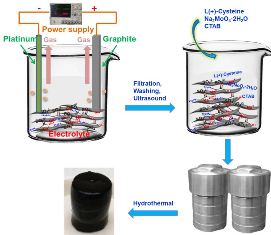
Scheme 1 Schematic illustration of the synthetic route of MoS<sub>2</sub>/NSGs-G composite.
