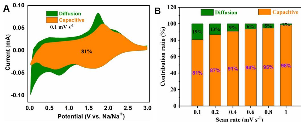
Fig. 5 Capacitive charge storage contribution (orange) and diffusion charge storage contribution (olive) at 0.1 mV s<sup>-1</sup> (A), normalized contribution ratio of capacitive (orange) and diffusion-controlled (olive) capacities at different sweep rates (B).
