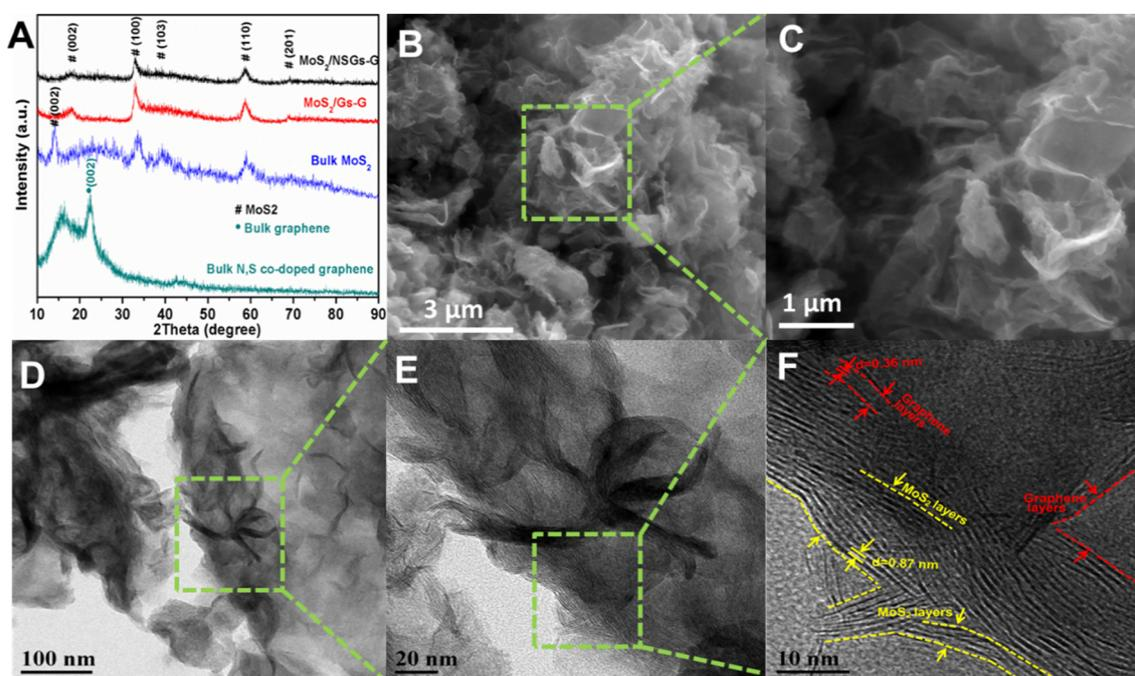
Fig. 1 XRD patterns of MoS<sub>2</sub>/NSGs-G, MoS<sub>2</sub>/Gs-G, bulk MoS<sub>2</sub> and bulk N, S-co-doped graphene (A), typical SEM (B and C), TEM and HRTEM images (D–F) of MoS<sub>2</sub>/NSGs-G sample.
