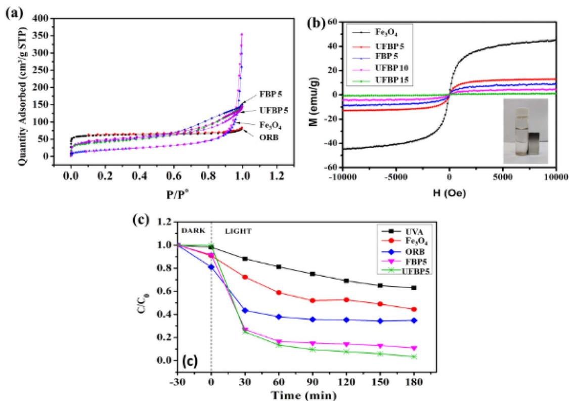
Fig. 5 (a) Nitrogen adsorption isotherms of ORB,  $\text{Fe}_3\text{O}_4$ , UFBP5, FBP5, (b) magnetization hysteresis loop of  $\text{Fe}_3\text{O}_4$ , FBP5, UFBP5, 10, 15 and (c) CIP photocatalytic degradation performance in the presence of UVA,  $\text{Fe}_3\text{O}_4$ , ORB, FBP5, UFBP5 under UVA, initial concentration  $10 \text{ mg L}^{-1}$ , pH 5.5,  $25^\circ\text{C}$ , rotation speed 300 rpm; inset in (b) is an image demonstrating the magnetic separation of UFBP5 from solution.
