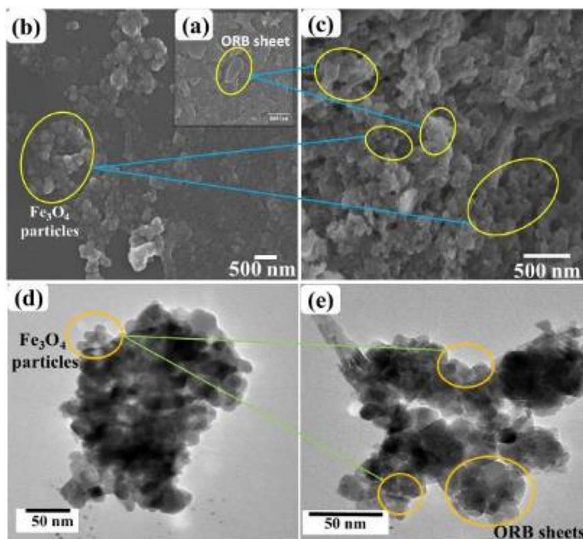
Fig. 3 (a–c) SEM images of ORB,  $\text{Fe}_3\text{O}_4$ , UFBP and (d, e) TEM images of  $\text{Fe}_3\text{O}_4$ , UFBP.
