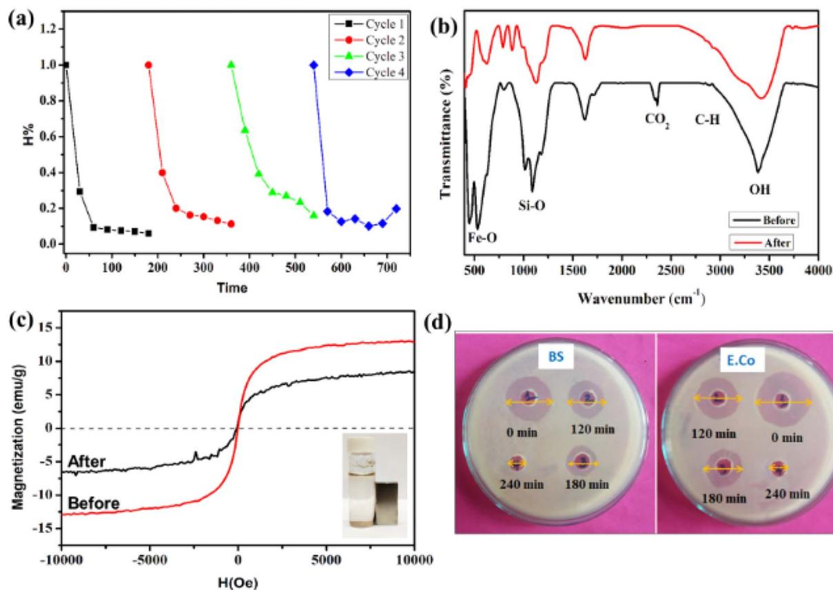
Fig. 9 (a) CIP photodegradation efficiency of reusing UFBP5 material, (b) FTIR and (c) VSM of UFBP5 before and after four recycle photo-degradation; (d) diameters of antibacterial zones *Bacillus subtilis* and (k) *Escherichia coli* at the different time of UVA illumination with the presence of UFBP5; inset in (c) is an image of UFBP5 magnetic separation from solution after 4<sup>th</sup> recycle.
