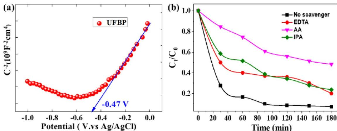
Fig. 6 (a) Mott-Schottky plots plotted as  $C^{-2}$  referenced to the Ag/AgCl electrode for UFBP; (b) photocatalytic degradation of CIP by UFBP under visible light irradiation and in the presence of scavengers: EDTA, AA, and IPA.
