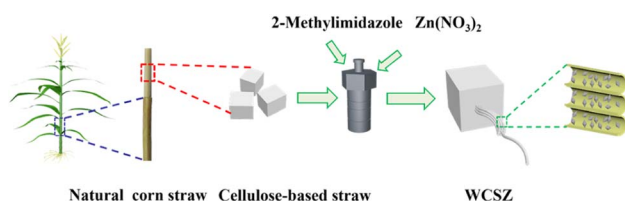
Fig. 1 Schematic of the fabrication of WCSZ composites.
