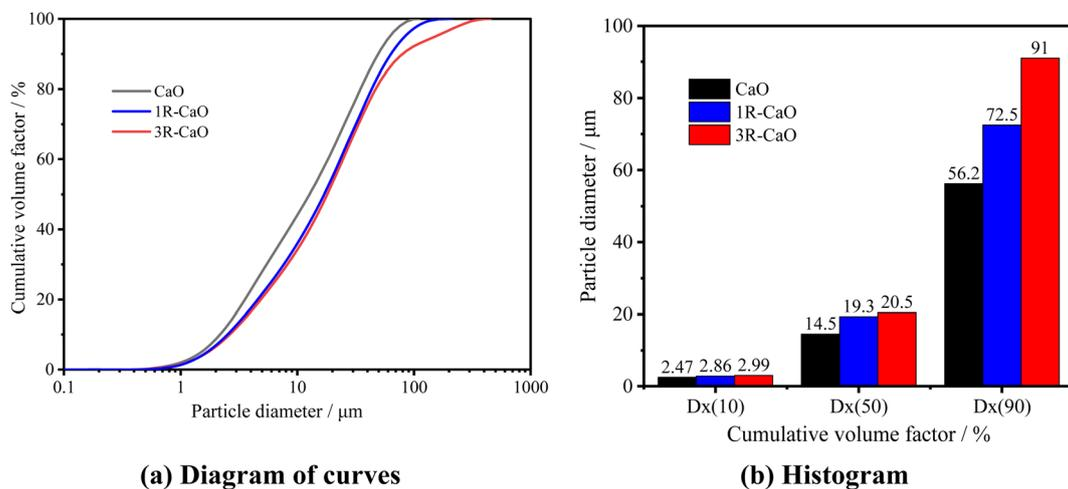
Fig. 6 Curves and histograms obtained for the pre-reaction cumulative particle size distributions of CaO, 1R-CaO, and 3R-CaO.
