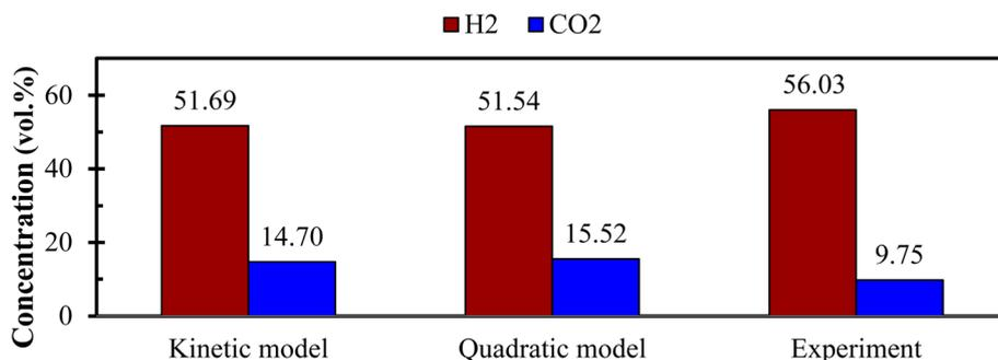
Fig. 7 Comparison of H<sub>2</sub> and CO<sub>2</sub> gas compositions between different models and experiment at optimum condition (ER = 0,  $d_p = 840 \mu\text{m}$ ,  $T = 1150 \text{ K}$ , SBR = 0.50).
