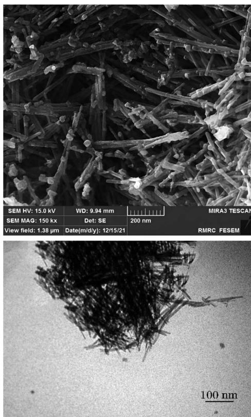
Fig. 8 FESEM (top) and TEM (bottom) images of the recovered catalyst after the 6<sup>th</sup> run.
