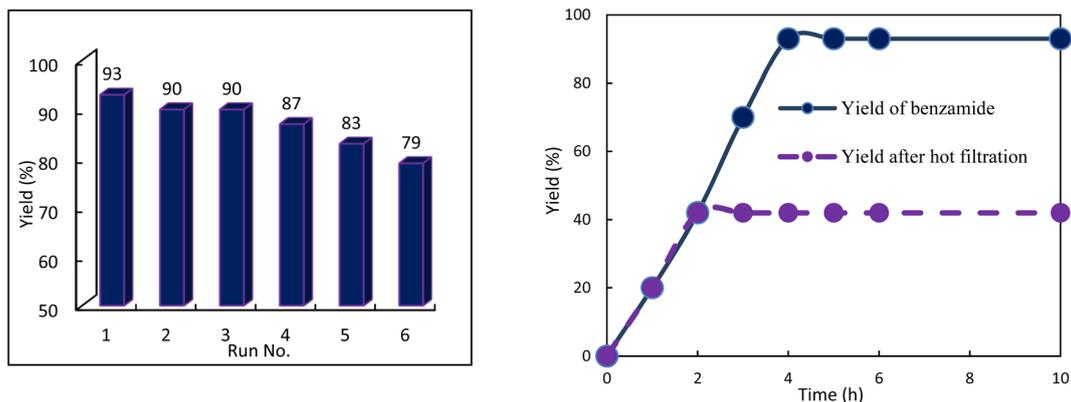
Fig. 7 (Left) Reusability of the Ag-OMS-2 for hydration of benzonitrile. (Right) The yield of benzamide in presence of Ag-OMS-2, and after its removal halfway.
