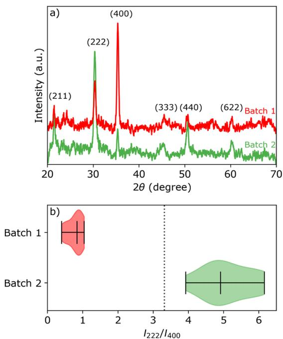
Fig. 1 (a)  $2\theta$  scans of representative batch 1 (red) and batch 2 (green) samples with the corresponding crystallographic orientations. (b) Violin plot of the peak intensity ratio distribution between the (222) and (400) peaks for samples from each batch. The distribution medians and limits are marked by the bars. The vertical dotted line represents the value of the theoretical ratio  $I_{222}/I_{400}$  for powder diffraction of  $\text{In}_2\text{O}_3$ .
