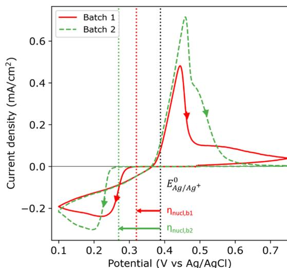
Fig. 2 First cycle of the cyclic voltammogram ( $25 \text{ mV s}^{-1}$ ) for the silver sulphate electrolyte containing saccharin on ITO batch 1 (red solid) and batch 2 (green dashed). The arrows indicate the scan direction. The nucleation onset potential is indicated with red and green dotted lines for batch 1 and 2, respectively. The black dotted line indicates the experimentally found Nernst equilibrium potential  $E_{\text{Ag}/\text{Ag}^+}^0$ .
