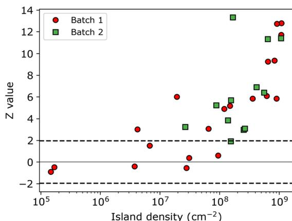
Fig. 6  $Z$ -Value obtained from individual nnd distributions as function of the island density. Samples from batch 1 and 2 are indicated by red circles and green squares, respectively. The black horizontal dashed lines indicates the region for which the distribution of islands exhibit CSR.
