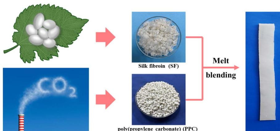
Fig. 2 Facile fabrication of shape-memory PPC/SF blend.
