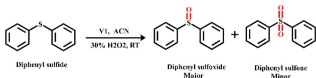
Scheme 5 \text{H}_2\text{O}_2 -assisted oxidation of diphenyl sulphide using V1 as a catalyst.
