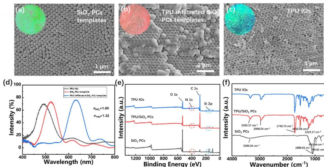
Fig. 5 Digital photos and SEM images of (a) SiO<sub>2</sub> PCs, (b) TPU/SiO<sub>2</sub> composite PCs and (c) TPU IOs, and (d) their corresponding reflected spectrums. (e) XPS spectrums and (f) FTIR spectrums of SiO<sub>2</sub> PCs, TPU/SiO<sub>2</sub> composite PCs and TPU IOs fabrics.
