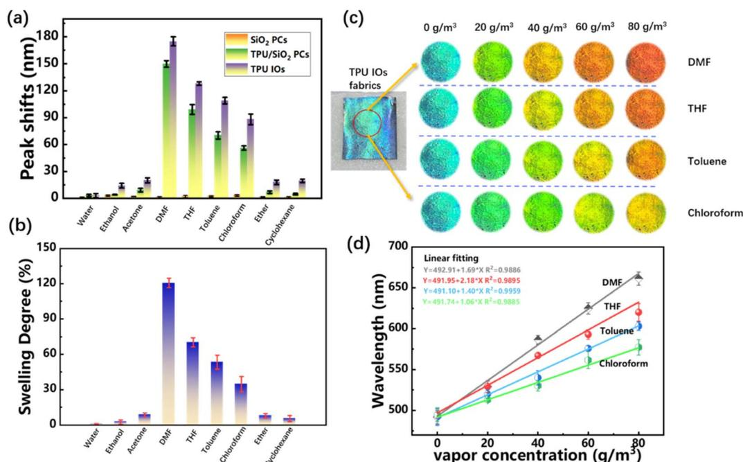
Fig. 7 (a) Reflected peak shifts of  $\text{SiO}_2$  PCs, TPU/ $\text{SiO}_2$  composite PCs and TPU IOs fabrics in various VOCs, (b) swelling degree of TPU film in various VOCs, (c) digital photos of TPU IOs fabrics in various concentrations of VOCs, (d) fitting curves of peak value and concentrations of VOCs.
