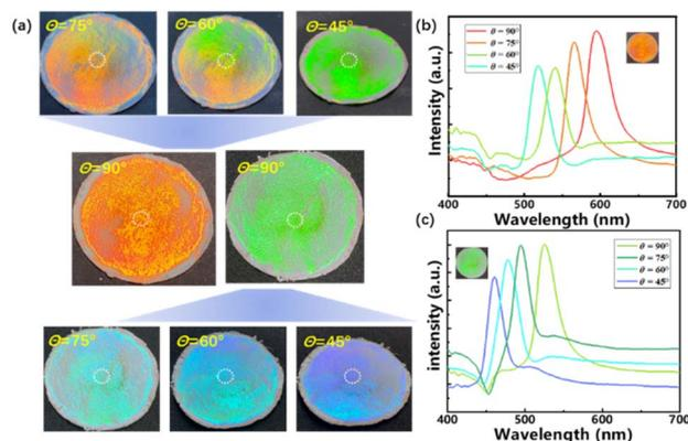
Fig. 3 Digital photos of SiO<sub>2</sub> PCs polyester fabrics with different particle sizes of (a) 357 nm and 258 nm and (b) and (c) changes in reflected peaks at different viewing angles from 90° to 45°.
