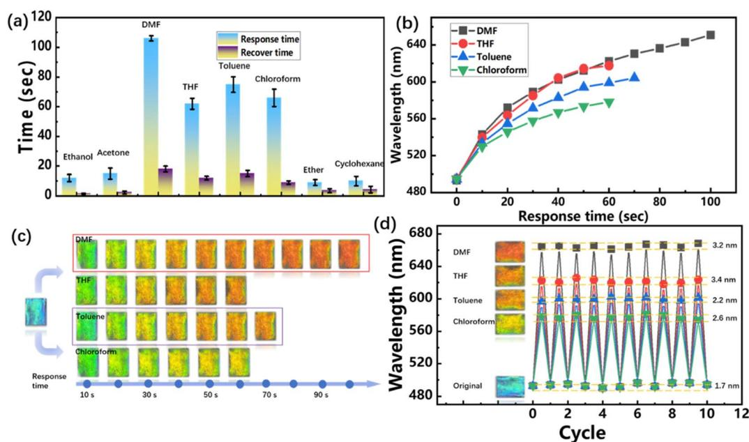
Fig. 8 (a) Response and recovery time of TPU IOs fabrics in various VOCs, (b) relationship between reflection peak and response time of TPU IOs fabrics, (c) digital photos of the response process of TPU IOs fabrics in DMF, THF, toluene, and chloroform, respectively, (d) the peak value of reflection spectrums and digital photos of TPU IOs fabrics after being alternately exposed to DMF, THF, toluene and chloroform vapor and air for 10 times.
