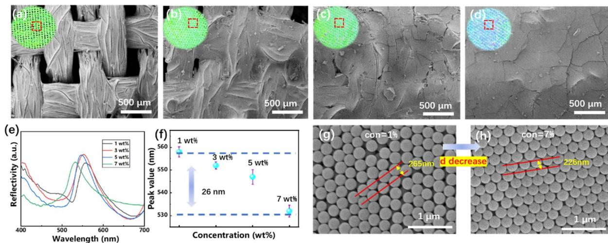
Fig. 1 Digital photos and SEM images of photonic crystal templates formed by (a) 1 wt%, (b) 3 wt%, (c) 5 wt%, (d) 7 wt% SiO<sub>2</sub> dispersion on the surface of polyester fabrics. (e) Reflection spectrums and (f) peak shifts of PCs polyester fabrics assembled by SiO<sub>2</sub> nanoparticle dispersions of different concentrations, SEM images of PCs assembled by (g) 1 wt% and (h) 7 wt% SiO<sub>2</sub> nanoparticle dispersions.
