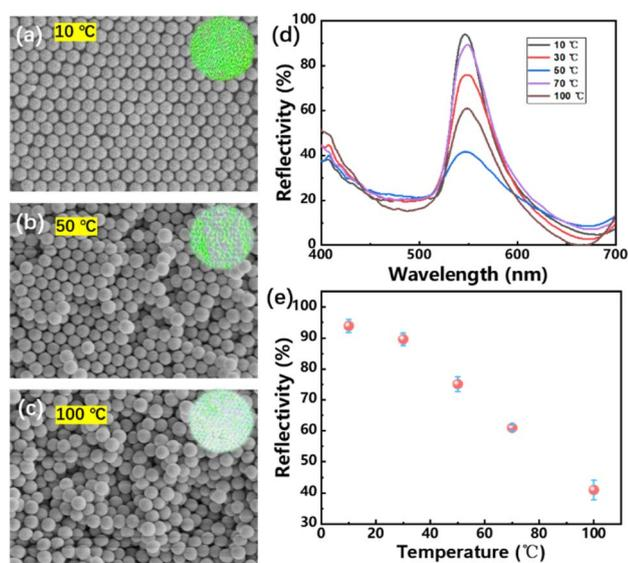
Fig. 2 SEM images and digital photos of PCs templates assembled by SiO<sub>2</sub> nanospheres at (a) 10, (b) 50, (c) 100 °C, corresponding (d) reflection spectrums and (e) change of peak intensity.
