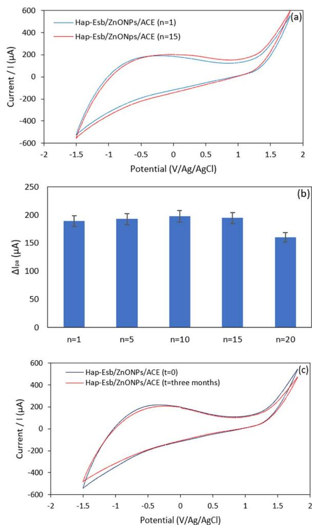
Fig. 8 (a) CV voltammograms of 0.1  $\mu\text{M}$  UA at  $n = 1$  and  $n = 15$  and (b) the histogram of oxidation peak current of 0.1  $\mu\text{M}$  UA at various repetitive measurement at Hap-Esb/ZnONPs/ACE; and (c) CV of UA measured using Hap-Esb/ZnONPs/ACE at different electrode stored for 0 and 3 months.
