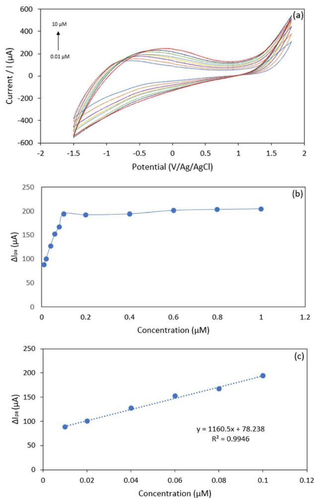
Fig. 7 (a) CV voltammogram of UA at 0.01–10  $\mu\text{M}$ ; (b) plot of UA concentration (0.01–1  $\mu\text{M}$ ) vs. anodic peak current; (c) plot of UA concentration (0.01–0.1  $\mu\text{M}$ ) vs. anodic peak current.
