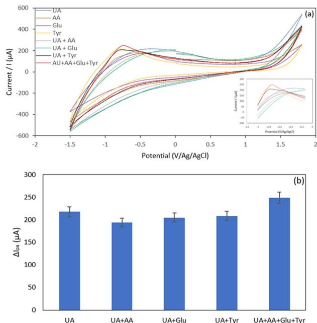
Fig. 9 (a) Voltammogram of 0.2  $\mu\text{M}$  interferent molecules on Hap-Esb/ZnONPs/ACE; (b) histogram of oxidation peak current of 0.2  $\mu\text{M}$  interferent molecules on Hap-Esb/ZnONPs/ACE.
