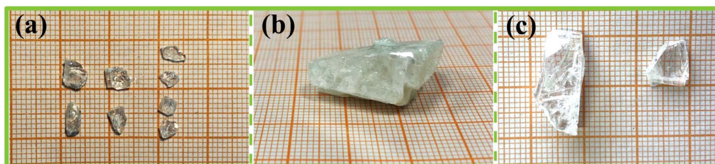
Fig. 3 (a) \text{Y}_2\text{Mo}_4\text{O}_{15} grains obtained by spontaneous crystallization; (b) seedless growth of \text{Y}_2\text{Mo}_4\text{O}_{15} single crystal; (c) photo of \text{Y}_2\text{Mo}_4\text{O}_{15} single crystal after optimizing seed crystal, flux system, and viscosity.
