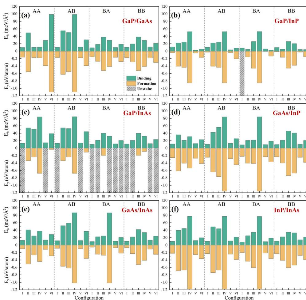
Fig. 3 The formation energies  $E_f$  (eV per atom) (yellow bars) and the binding energies  $E_b$  ( $\text{meV } \text{\AA}^{-2}$ ) (green bars) for the configurations of (a) GaP/GaAs, (b) GaP/InP, (c) GaP/InAs, (d) GaAs/InP, (e) GaAs/InAs, and (f) InP/InAs heterostructures. The structures with positive formation energies are considered unstable and marked with grey bars.
