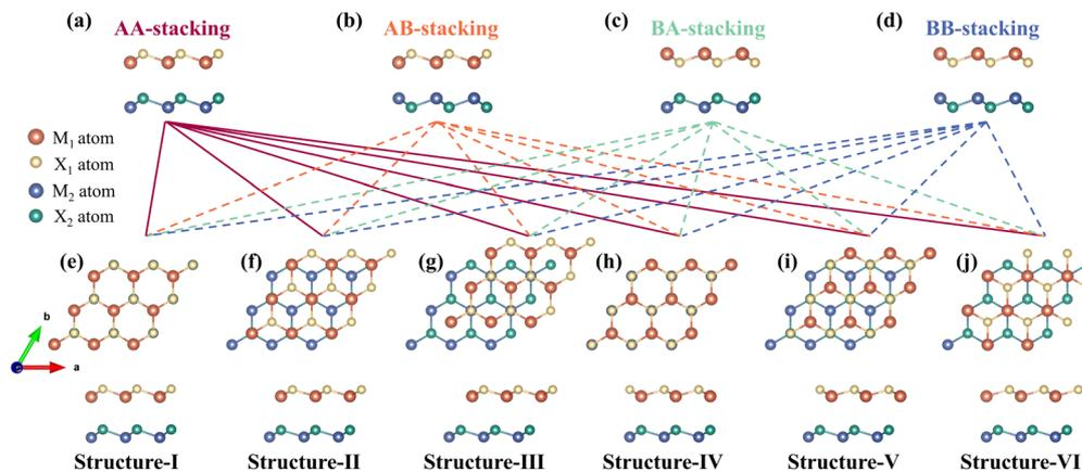
Fig. 2 (a)–(d) The side views of 4 different stacking models for the  $M_1X_1/M_2X_2$  heterostructure. (e)–(j) The top and side views of the 6 possible structures of each stacking model with AA-stacking as an example. A total of 144 different configurations are achieved (with 24 configurations for each  $M_1X_1/M_2X_2$  heterostructure).
