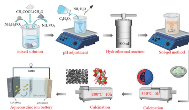
Fig. 1 The illustration of synthesis processes for \text{Li}_3\text{V}_2(\text{PO}_4)_3 cathode materials.
