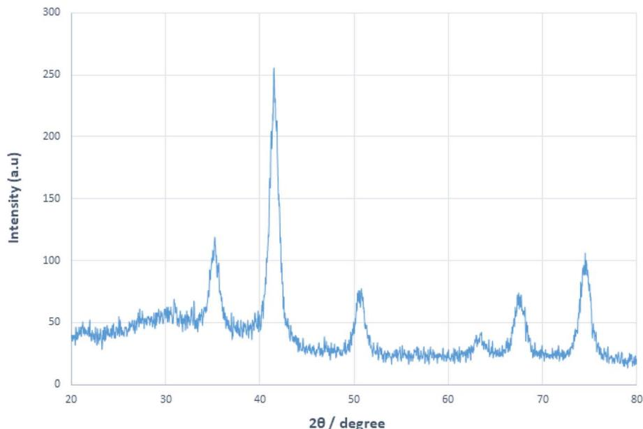
Fig. 10 XRD analysis of MNP-[Dop-OH]-CuBr<sub>2</sub> nanocatalysts after 8 runs.
