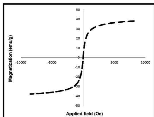
Fig. 11 VSM analysis of MNP-[Dop-OH]-CuBr<sub>2</sub> nanocatalysts after 8 runs.
