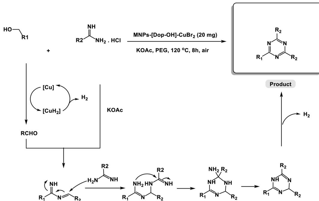
Scheme 2 Suggested mechanism for the oxidative coupling reaction of amidine hydrochlorides and alcohols catalyzed by MNP-[Dop-OH]-CuBr<sub>2</sub> nanocomposites under air conditions.
