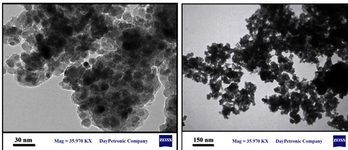
Fig. 4 TEM images of MNP-[Dop-OH]-CuBr<sub>2</sub> nanocatalysts at different magnifications.
