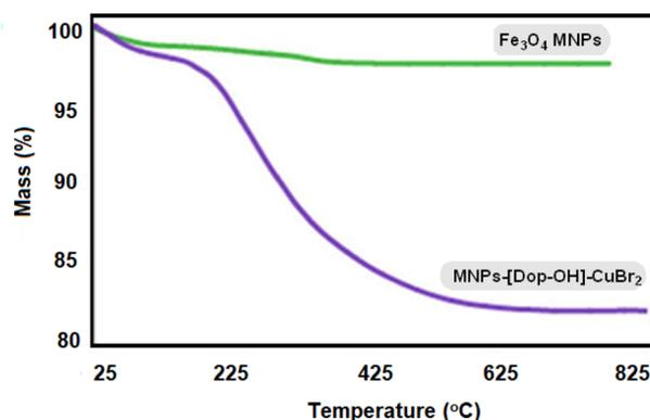
Fig. 8 TGA analysis of Fe<sub>3</sub>O<sub>4</sub> MNPs and MNP-[Dop-OH]-CuBr<sub>2</sub> nanocatalysts.
