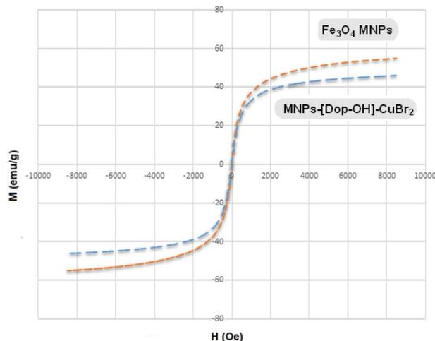
Fig. 7 VSM analysis of Fe<sub>3</sub>O<sub>4</sub> MNPs and MNP-[Dop-OH]-CuBr<sub>2</sub> nanocatalysts.
