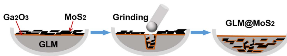
Fig. 1 Schematic presentation of preparation process of GLM@MoS 2 . Initially, the GLM is surrounded by Ga 2 O 3 oxides and separated from MoS 2 nanosheets. Then the grinding process make MoS 2 nanosheets disperse into GLM by the adhesion property of Ga 2 O 3 . And finally the GLM@MoS 2 composite is obtained.
