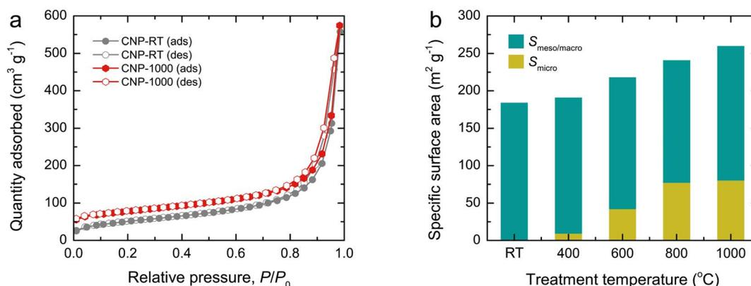
Fig. 4 (a) N<sub>2</sub> adsorption–desorption isotherms and (b) bar plots showing the contribution of specific surface area ( $S_{\text{BET}}$ ) of CNPs by micropores ( $S_{\text{micro}}$ ) and meso–macropores ( $S_{\text{meso/macro}}$ ).
