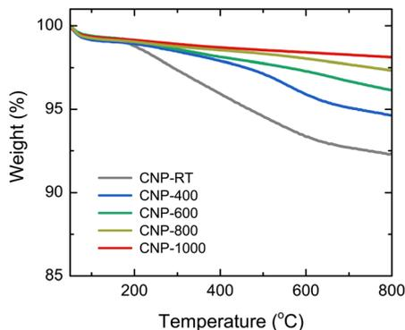
Fig. 3 TGA curves of CNPs in the temperature range of 50 to 800 °C under an N<sub>2</sub> flow.
