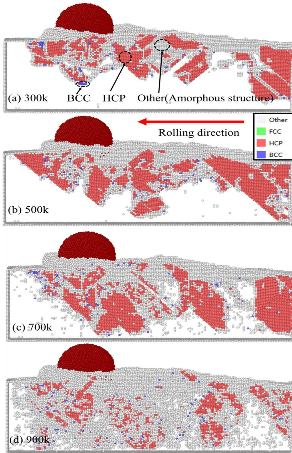
Fig. 9 Schematic diagram of defect atom distribution.
