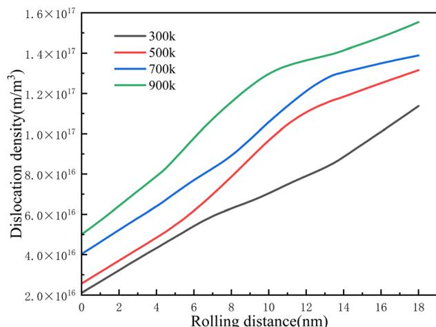
Fig. 7 Dislocation density at different rolling temperatures.
