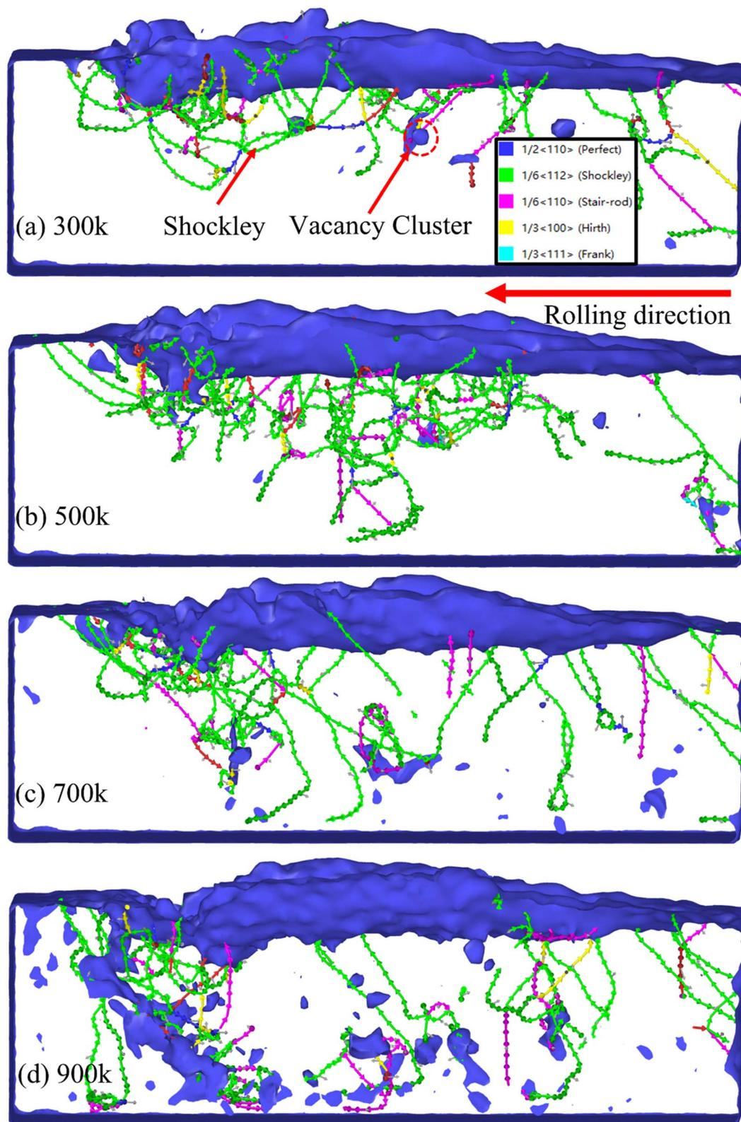
Fig. 8 Dislocation type distribution diagram.
