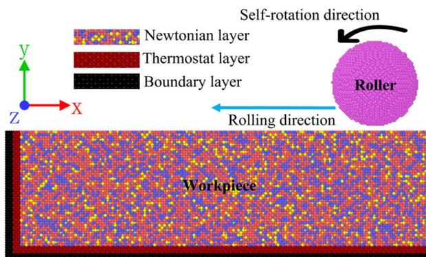
Fig. 1 Rolling model diagram.
