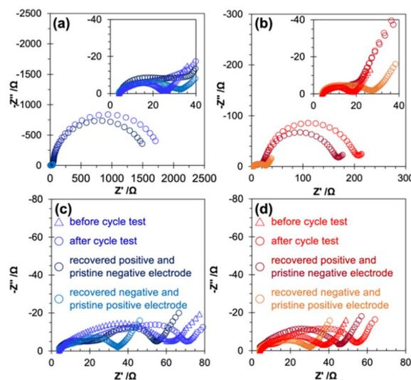
Fig. 5 Electrochemical impedance spectra for cells with recovered and pristine electrodes in (a) PFP-F<sub>2</sub>, (b) HHIB-F<sub>2</sub>, (c) PFP-F<sub>2</sub> with LiBOB, and (d) HHIB-F<sub>2</sub> with LiBOB. Each legend represents the conditions of the cell for EIS measurements.
