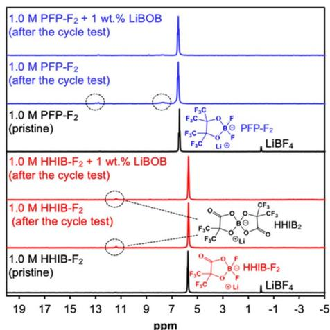
Fig. 3  $^{11}\text{B}$ -NMR spectra of pristine electrolytes and electrolytes extracted from the cycle tested cell.  $\text{LiBF}_4$  at 0 ppm is an internal standard added to the pristine PFP- $\text{F}_2$  and HHIB- $\text{F}_2$  samples. The  $\text{LiBF}_4$  internal standard was not added to the electrolytes extracted from cycle tested cell to avoid the overlap with the generated  $\text{LiBF}_4$  via the decomposition of PFP- $\text{F}_2$  and HHIB- $\text{F}_2$  during the cycle test.
