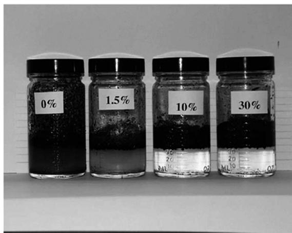
Fig. 7 30%, 1.5% and 0%  $\text{CF}_3$ -aerogels mixed with Prudhoe Bay crude oil with 3 wt% NaCl Reynold *et al.*, *J. Non-Cryst. Solids*, 2001.<sup>67</sup>
