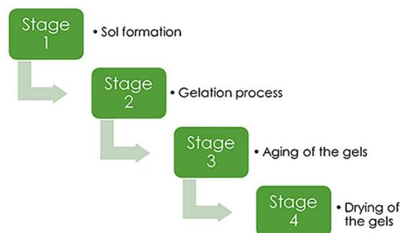
Fig. 2 Main stages of aerogel synthesis, Gahramanli et al., ISPC KOGF-2022.<sup>43</sup>
