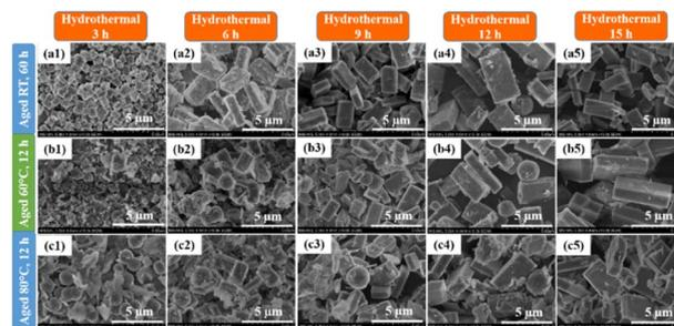
Fig. 7 SEM images of ZSM-5 crystal at various crystallization conditions.
