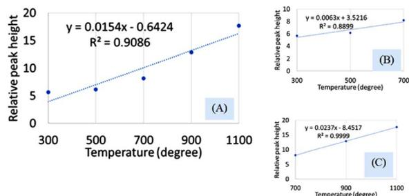
Fig. 3 Dependency of relative peak intensity on the sintering temperature for (A) 300–1100 °C temperature, (B) 300–700 °C temperature, and (C) 700–1100 °C temperature.
