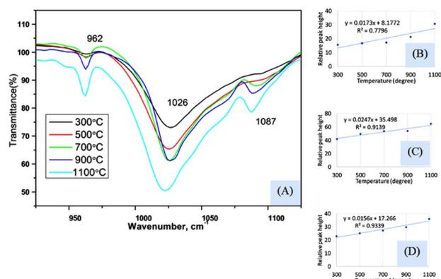
Fig. 4 (A) FTIR spectrum in the range of 925–1125  $\text{cm}^{-1}$ , (B) relation between temperature and relative peak height for 962  $\text{cm}^{-1}$  wavenumber, (C) relation between temperature and relative peak height for 1026  $\text{cm}^{-1}$  wavenumber, and (D) relation between temperature and relative peak height for 1087  $\text{cm}^{-1}$  wavenumber.
