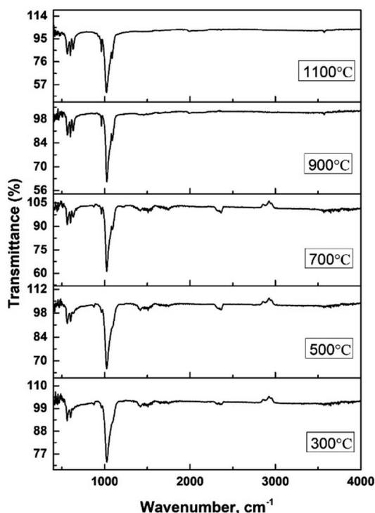
Fig. 1 FTIR of synthesized amorphous and crystalline hydroxyapatite.
