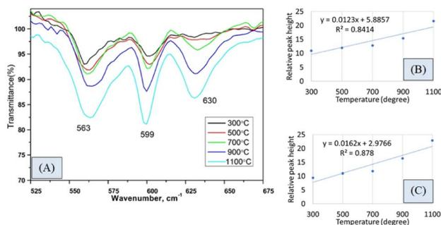
Fig. 2 (A) FTIR spectrum in the range of 525–675  $\text{cm}^{-1}$ , (B) relation between temperature and relative peak height for 563  $\text{cm}^{-1}$  wavenumber, and (C) relation between temperature and relative peak height for 599  $\text{cm}^{-1}$  wavenumber.
