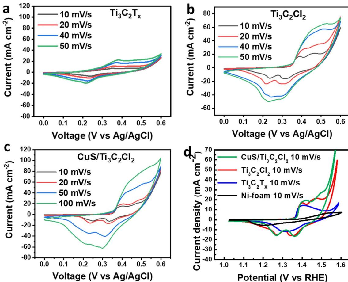
Fig. 6 (a) Cyclic voltammetry (CV) analysis of hydrofluoric acid (HF) based MXene ( $\text{Ti}_3\text{C}_2\text{T}_x$ ) at different scan rates, (b) CV analysis of Cl-terminated MXene ( $\text{Ti}_3\text{C}_2\text{Cl}_2$ ) at different increasing scan rates, (c) CV analysis of CuS/Cl-terminated MXene ( $\text{CuS}/\text{Ti}_3\text{C}_2\text{Cl}_2$ ) composite at different scan rates, (d) comparison of CV of Ni foam, HF-MXene, Cl-MXene and CuS/Cl-MXene at  $10 \text{ mV s}^{-1}$  scan rate.
