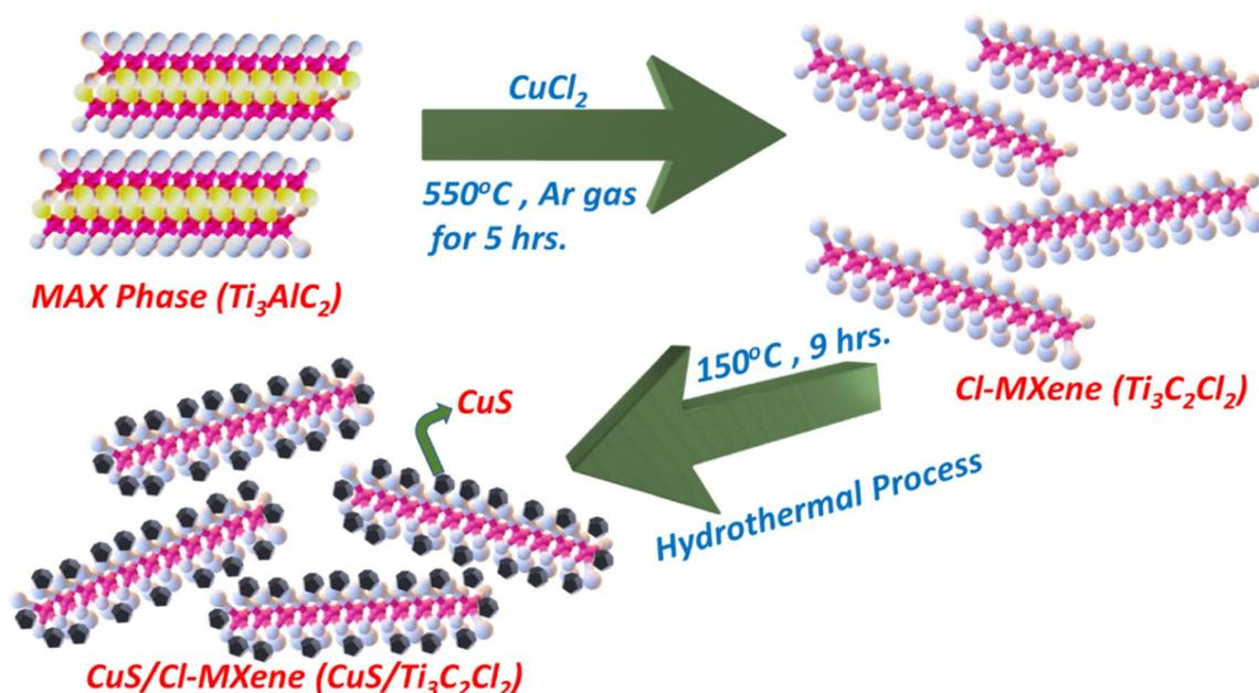
Fig. 1 Schematic illustration of the synthesis of Cl-terminated MXene from the heat treatment procedure of MAX phase ( $\text{Ti}_3\text{AlC}_2$ ) and copper chloride ( $\text{CuCl}_2$ ), then deposition of CuS nano particles on Cl-MXene sheets by hydrothermal process.
