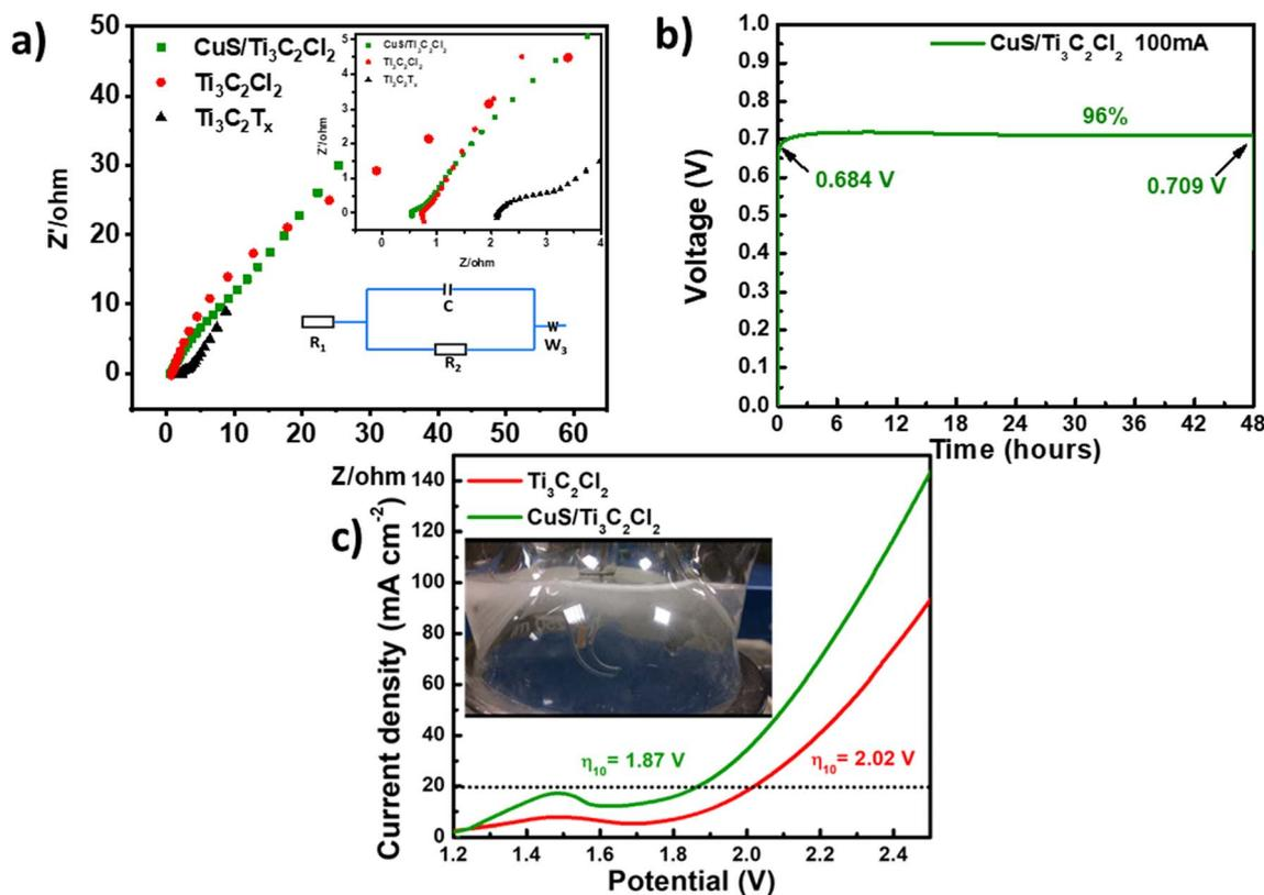
Fig. 7 (a) Electrochemical impedance spectroscopy (EIS) analysis of HF-MXene ( $\text{Ti}_3\text{AlC}_2$ ), Cl-MXene ( $\text{Ti}_3\text{C}_2\text{Cl}_2$ ) and CuS/Cl-MXene ( $\text{CuS}/\text{Ti}_3\text{C}_2\text{Cl}_2$ ), (b) chronopotentiometry (CP) analysis of synthesized CuS/Cl-MXene ( $\text{CuS}/\text{Ti}_3\text{C}_2\text{Cl}_2$ ), (c) overall water splitting curves of both Cl-MXene ( $\text{Ti}_3\text{C}_2\text{Cl}_2$ ) and CuS/Cl-MXene ( $\text{CuS}/\text{Ti}_3\text{C}_2\text{Cl}_2$ ).
