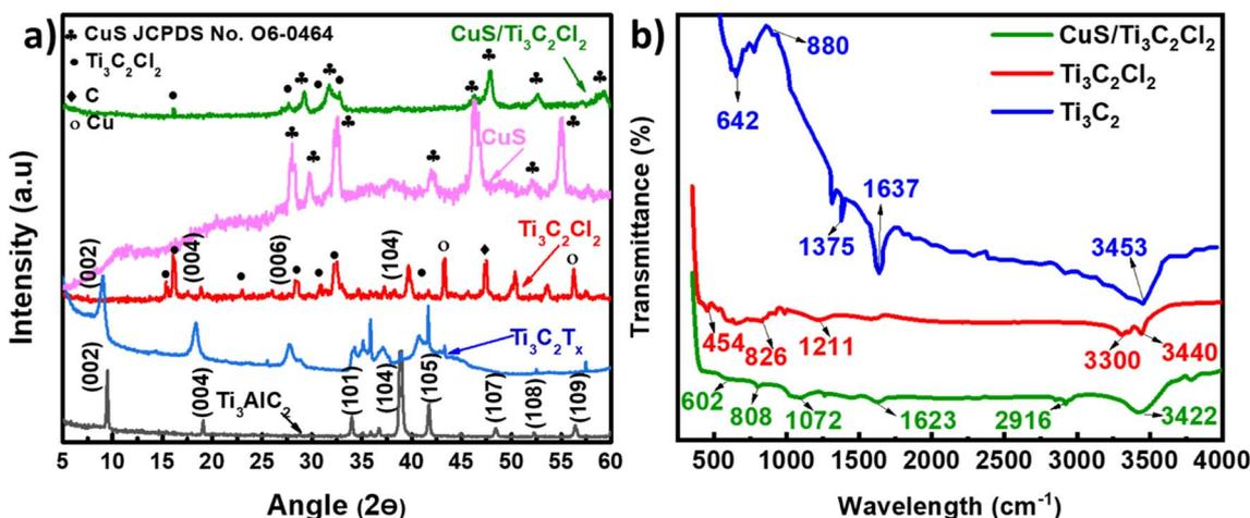
Fig. 4 (a) XRD analysis of MAX phase (Ti<sub>3</sub>AlC<sub>2</sub>), HF-MXene (Ti<sub>3</sub>C<sub>2</sub>T<sub>x</sub>), Cl-MXene (Ti<sub>3</sub>C<sub>2</sub>Cl<sub>2</sub>), CuS and composite CuS/Ti<sub>3</sub>C<sub>2</sub>Cl<sub>2</sub>, (b) FTIR spectrum of HF-MXene (Ti<sub>3</sub>C<sub>2</sub>T<sub>x</sub>), Cl-MXene (Ti<sub>3</sub>C<sub>2</sub>Cl<sub>2</sub>) and CuS/Cl-MXene (CuS/Ti<sub>3</sub>C<sub>2</sub>Cl<sub>2</sub>).
