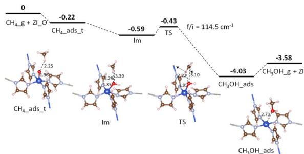
Fig. 6 Potential energy surface for CH<sub>4</sub> conversion over Zl<sub>2</sub>O via the CH<sub>4</sub>\_ads\_t pathway. Relative energies are given in eV. The zero-reference energy is the sum of the total energies of the isolated CH<sub>4</sub> molecule and Zl<sub>2</sub>O. Zero-point energy correction is not included.
