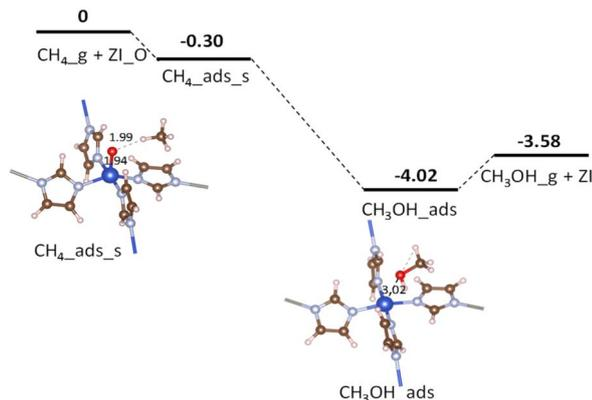
Fig. 5 Potential energy surface for CH<sub>4</sub> oxidation over ZI\_O via the CH<sub>4</sub>\_ads\_s pathway. Relative energies are given in eV. The zero-reference energy is the sum of the total energies of the isolated CH<sub>4</sub> molecule and ZI\_O. Zero-point energy correction is not included.
