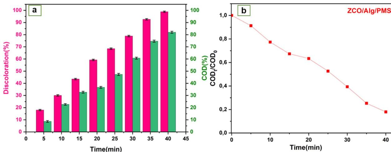
Fig. 8 (a and b) Analysis of chemical oxygen demand (COD) versus time using ZCO/Alg catalyst under the conditions, [catalyst] = 1 g l<sup>-1</sup>, [RhB] = 25 mg l<sup>-1</sup>, [PMS] = 1 g l<sup>-1</sup>, ambient temperature.
