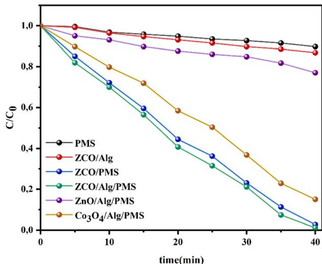
Fig. 5 degradation of RhB solutions in various systems. Initial concentrations: [RhB] = 25 mg l<sup>-1</sup>, [catalyst] = 1 g l<sup>-1</sup>, [PMS] = 1 g l<sup>-1</sup>, ambient temperature.
