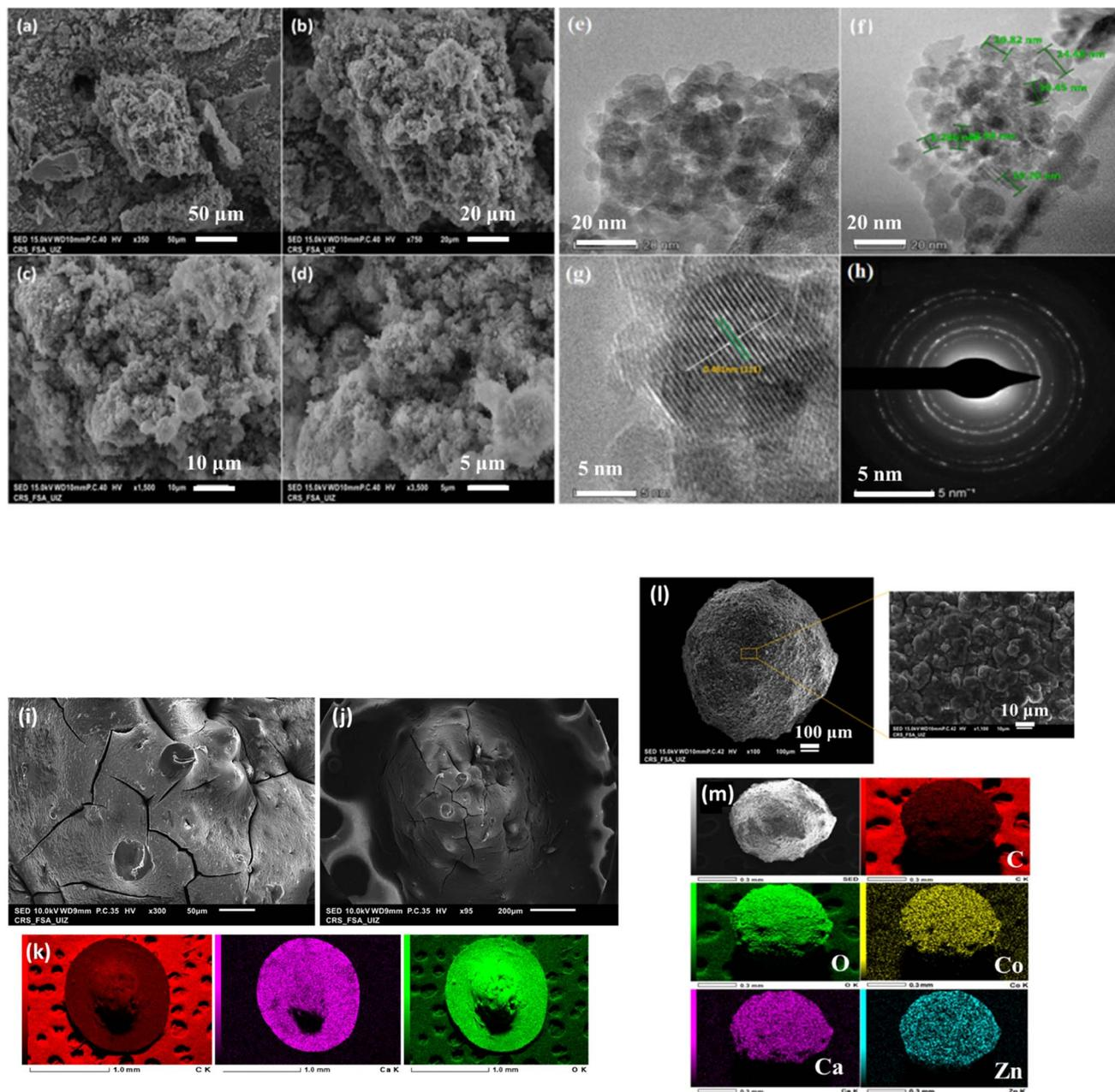
Fig. 3 (a–d) SEM images of  $\text{ZnCo}_2\text{O}_4$  powder at different resolution. TEM (e and f) and (g) HR-TEM images of  $\text{ZnCo}_2\text{O}_4$  powder, and (h) SAED pattern. (i–k) SEM images and mapping of Alg beads. (l and m) SEM images and mapping of Alg/ZCO beads.
