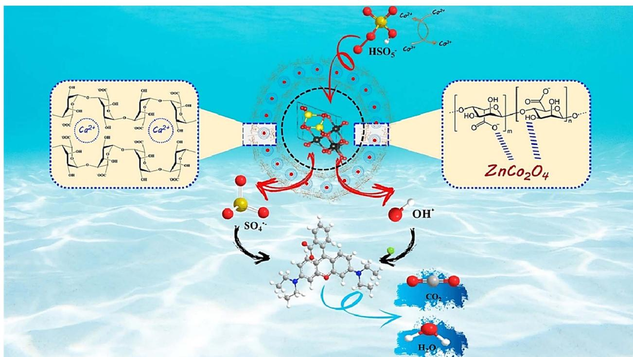
Scheme 1 Mechanism of peroxymonosulfate (PMS) activation on ZCO@Alg.
