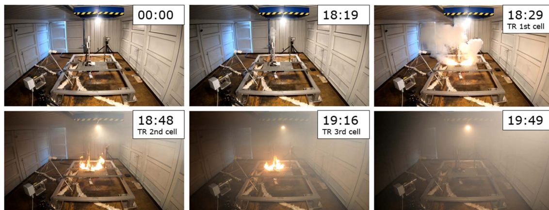
Fig. 5 Progress of three-cell stack test (test #06, time after start of the test).
