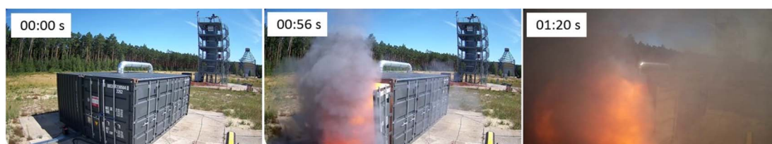
Fig. 13 Test #09, subsequent gas explosion due TR and pressure release of the experimental room.
