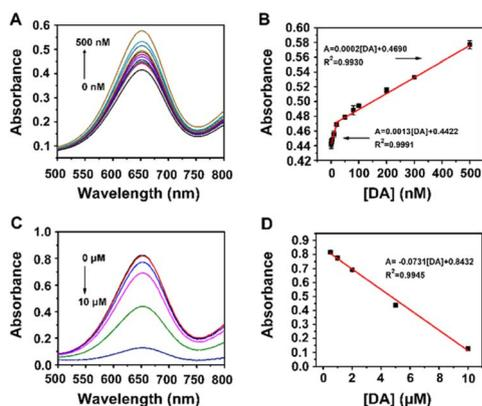
Fig. 3 (A) UV-vis spectra and (B) absorbance response of  $\text{MoS}_2\text{-MIL-101(Fe)}\text{-H}_2\text{O}_2\text{-TMB}$  system in different concentrations of DA in the “signal-on” mode. (C) UV-vis spectra and (D) absorbance response of  $\text{MoS}_2\text{-MIL-101(Fe)}\text{-H}_2\text{O}_2\text{-TMB}$  system in different concentrations of DA in the “signal-off” mode.
