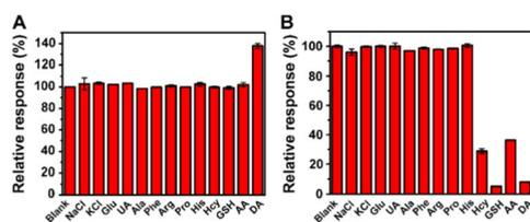
**Fig. 4** (A) Selectivity experiment of the "signal-on" mode to DA and various substances at 0.5  $\mu\text{M}$ . (B) Selectivity experiment of the "signal-off" mode to DA and various substances at 50  $\mu\text{M}$ .
