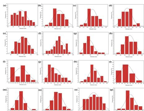
**Fig. 3** Diameter distribution of PVA/CS/erythromycin composite nanofibers in (a) 50/50, (b) 70/30 and (c) 100/0 volume ratio of PVA/CS, (d) 1%, (e) 2%, (f) 5%, (g) 10% and (h) 20% of erythromycin, (i) 5, (j) 10, (k) 15 and (l) 20 kV of high voltage, and (m) 10, (n) 15, (o) 18 and (p) 20 cm for nozzle to drum distance.
