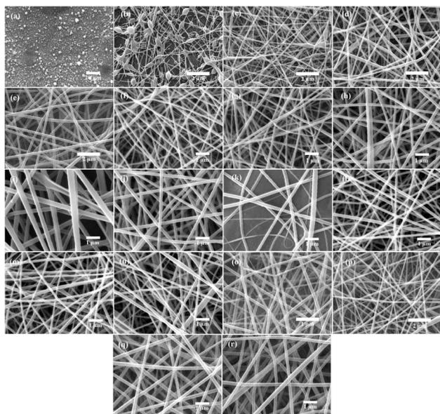
**Fig. 2** The SEM image of PVA/CS/erythromycin composite nanofibers in (a) 0/100, (b) 30/70, (c) 50/50, (d) 70/30 and (e) 100/0 volume ratio of PVA/CS, (f) 1%, (g) 2%, (h) 5%, (i) 10% and (j) 20% of erythromycin, (k) 5, (l) 10, (m) 15 and (n) 20 kV of high voltage, and (o) 10, (p) 15, (q) 18 and (r) 20 cm for nozzle to drum distance.
