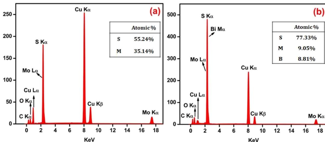
Fig. 5 (a and b) EDAX spectra of the pristine MoS<sub>2</sub> and MBS-4 nanocomposite.
