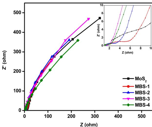
**Fig. 11** Nyquist plot of pristine MoS<sub>2</sub> and MoS<sub>2</sub>/Bi<sub>2</sub>S<sub>3</sub> nanocomposites.
