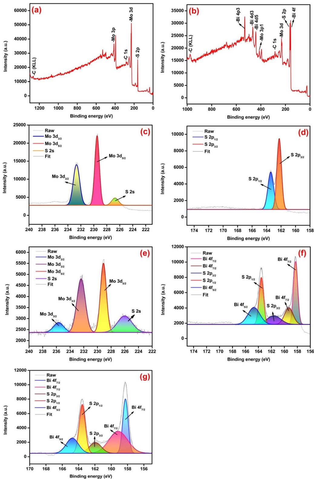
Fig. 6 (a and b) Survey spectrum of pristine MoS<sub>2</sub> and MoS<sub>2</sub>/Bi<sub>2</sub>S<sub>3</sub> nanocomposite, (c and d) XPS spectra of pristine MoS<sub>2</sub> for Mo 3d and S 2p respectively, (e–g) XPS spectra of MBS-4 nanocomposite for Mo 3d, S 2p and Bi 4f, respectively.
