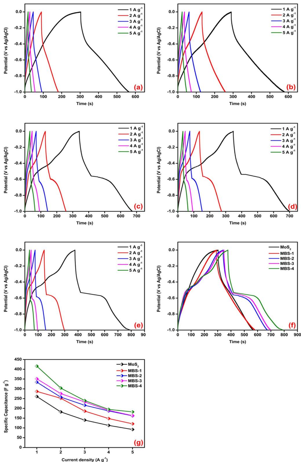
Fig. 9 (a–e) Charge–discharge characteristics of pristine MoS<sub>2</sub>, MBS-1, MBS-2, MBS-3, and MBS-4 nanocomposites, respectively, (f) comparison of charge–discharge characteristics of pristine MoS<sub>2</sub> and MoS<sub>2</sub>/Bi<sub>2</sub>S<sub>3</sub> nanocomposites at a current density of 1 A g<sup>-1</sup>, (g) specific capacitances of pristine MoS<sub>2</sub> and MoS<sub>2</sub>/Bi<sub>2</sub>S<sub>3</sub> nanocomposites at various current densities by charge–discharge analysis.
