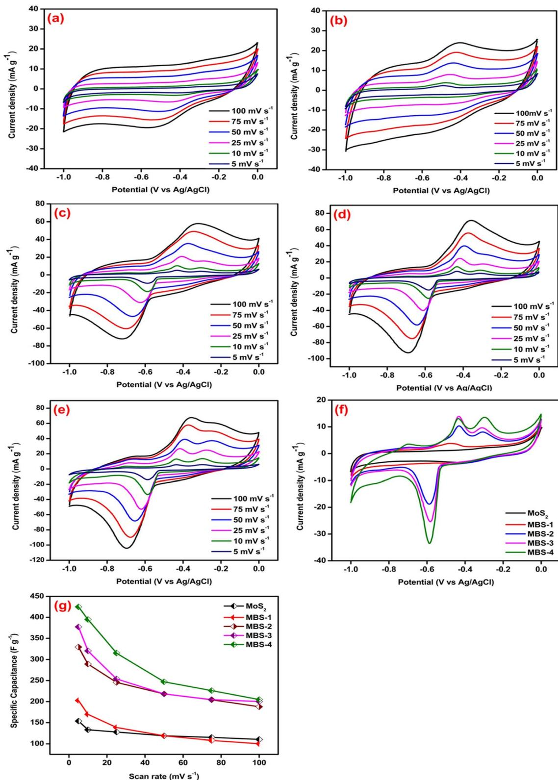
Fig. 7 (a–e) Cyclic voltammetry curves of pristine MoS<sub>2</sub>, MBS-1, MBS-2, MBS-3, and MBS-4 electrodes, respectively (f) comparison of CV curves of pristine MoS<sub>2</sub> and MoS<sub>2</sub>/Bi<sub>2</sub>S<sub>3</sub> nanocomposites at a scan rate of 5 mV s<sup>-1</sup>, (g) specific capacitances of pristine MoS<sub>2</sub> and MoS<sub>2</sub>/Bi<sub>2</sub>S<sub>3</sub> nanocomposites at various scan rates by cyclic voltammetry analysis.
