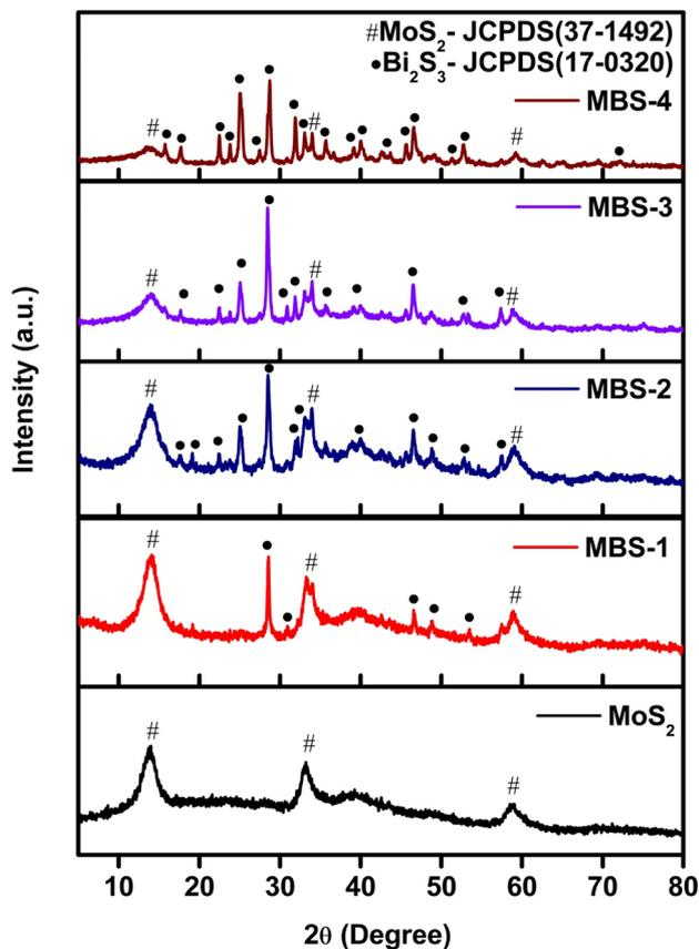
Fig. 2 XRD patterns of the pristine MoS<sub>2</sub>, MBS-1, MBS-2, MBS-3, and MBS-4 samples.
