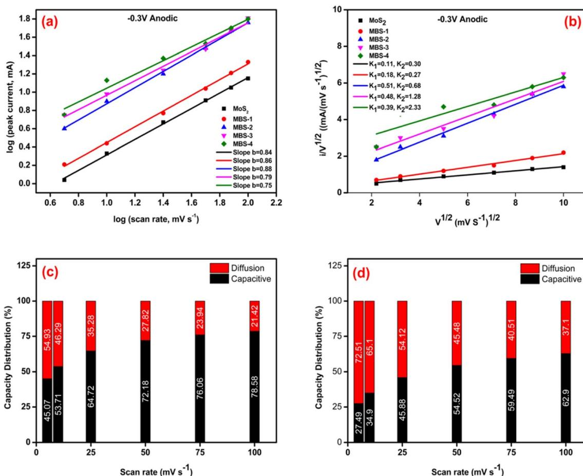
**Fig. 8** (a–d) Capacitive charge storage distribution calculation, (a) power law ( $i = av^b$ ) dependence of current on sweep rate for MoS<sub>2</sub> and MoS<sub>2</sub>/Bi<sub>2</sub>S<sub>3</sub> composites, (b) response of  $v^{1/2}$  vs.  $i/v^{1/2}$  (c) comparison of the capacitive and diffusion capacities distribution for MoS<sub>2</sub> electrode, (d) comparison of the capacitive and diffusion capacities distribution for MBS-4 electrode.
