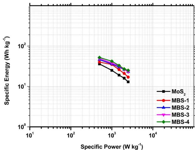
**Fig. 10** Ragone plot of pristine MoS<sub>2</sub> and MoS<sub>2</sub>/Bi<sub>2</sub>S<sub>3</sub> nanocomposites.
