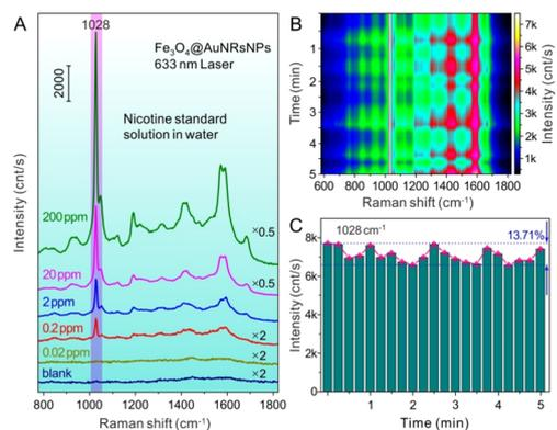
Fig. 3 (A) A series of SERS spectra of nicotine in water at different concentrations with  $\text{Fe}_3\text{O}_4@AuNRsNPs$  as the SERS substrates combined with a capillary, respectively. (B) Time-dependent SERS spectra of 20 ppm nicotine based on  $\text{Fe}_3\text{O}_4@AuNRsNPs$  combined with a capillary. (C) Time-dependent SERS intensity fluctuation of nicotine based on  $\text{Fe}_3\text{O}_4@AuNRsNPs$  substrates combined with a capillary.
