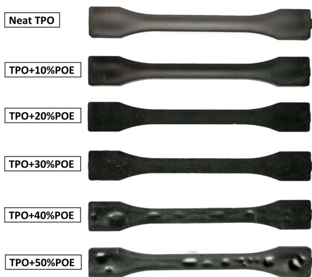
Fig. 6 Injection-moulded tensile specimens of TPO and TPO-POE blends, 4 mm thickness, showing sink mark defects on the surface of TPO + 40%POE and TPO + 50%POE specimens.
