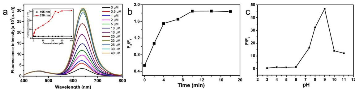
Fig. 4 (a) Fluorescence spectra of the CQDs/CdTe QDs system in the presence of different concentrations of Cd<sup>2+</sup> (the inset showed the fluorescence intensity of CQDs (black) and CdTe QDs (red)). (b) Curve of  $F_2/F_1$  under different recovery times, where  $F_2$  and  $F_1$  represent the FL values of CQDs and CdTe QDs, respectively. (c) Curve of  $F/F_0$  under different pH, where  $F$  and  $F_0$  represent the FL values of CdTe QDs before and after adding Cd<sup>2+</sup>.
