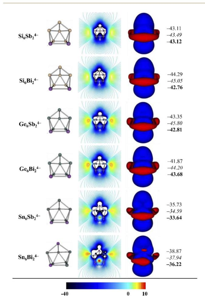
Fig. 4 Isosurface and contour plot for  $B_z^{\text{ind}}$  and the external field (NICS<sub>zz</sub>). The isosurface value is set to  $\pm 3.0$  ppm. Blue: long range shielding regions; red: deshielding regions.  $B_z^{\text{ind}}$  values at the cage center are reported at the PBE0/def2-TZVP, PBE0-ZORA/TZ2P (italic) and PBE0-SO/TZ2P (bold) levels.
