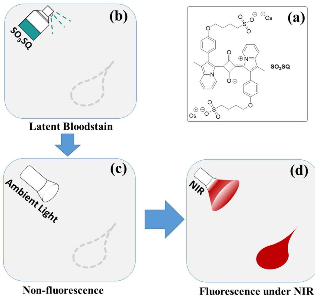
**Scheme 1** The principle for visualization of latent bloodstain: (a) the chemical structure of  $\text{SO}_3\text{SQ}$ ; (b) latent bloodstain pattern; (c) non-fluorescent  $\text{SO}_3\text{SQ}$  under ambient light; (d) visualization of the bloodstain under NIR light.
