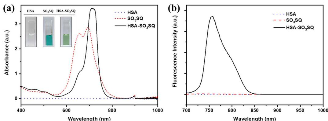
Fig. 1 (a) Absorption and (b) emission spectra of pure HSA (5.0 mg mL<sup>-1</sup>), pure  $\text{SO}_3\text{SQ}$  (0.075 mg mL<sup>-1</sup>) and the mixture of HSA with  $\text{SO}_3\text{SQ}$  in aqueous solution. The excitation wavelength is 693 nm. Inset is the photograph for three solutions.
