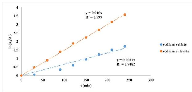
Fig. 1 Effect of the supporting electrolyte on the PS dye degradation using the EF process. Experimental conditions: [PS] = 0.06 mM; [Fe<sup>2+</sup>] = 0.12 mM; [supporting electrolyte] = 0.2 mM; T = 25 °C; pH = 3.34.
