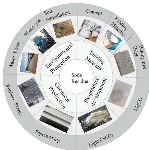
Fig. 2 Soda residue resource utilization.
