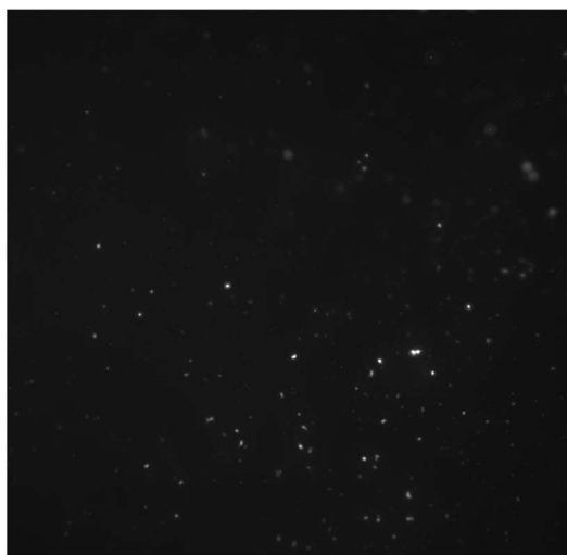
Fig. 8 Fluorescence microscope image of sol-gel glass with CdSe/CdS nanoparticles.
