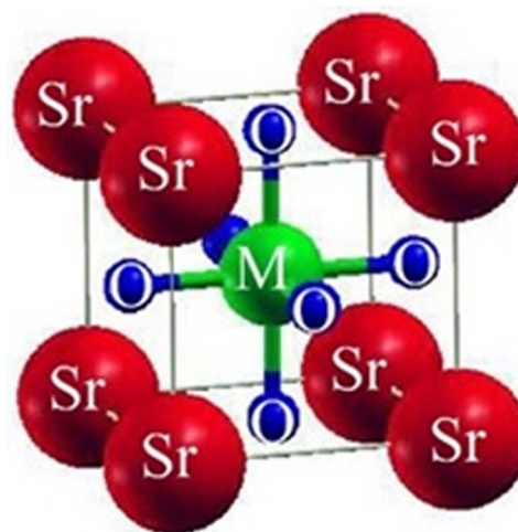
Fig. 1 The conventional cubic crystal structure of ternary molecules SrMO 3 (M = Hf, Pt).
