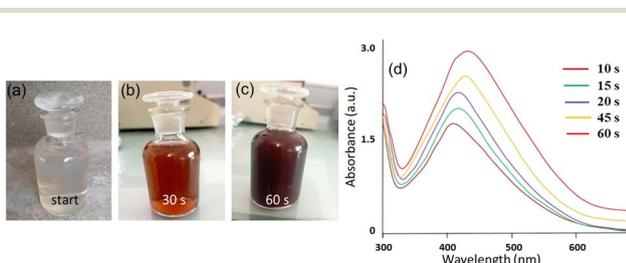
Fig. 2 Photographs of 1 mM  $\text{AgNO}_3$  + ED extract mixture after exposure to sunlight for (a) 0 s (start), (b) 30 s, and (c) 60 s showing color changes with time. (d) UV-vis spectra of ED-AgNPs suspension after different reaction times.
