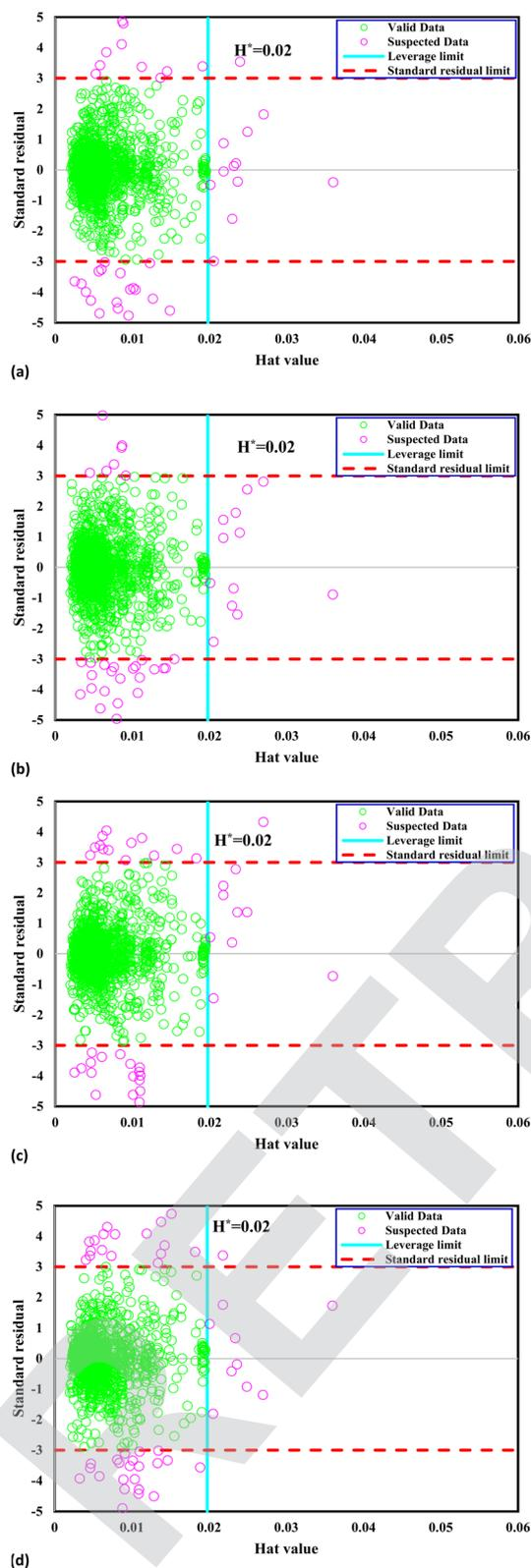
Fig. 1 William's plot of the CO<sub>2</sub> solubility data bank to find outliers for Kernel-based GPR model of (a) Matern, (b) exponential, (c) squared exponential, (d) rational quadratic.
