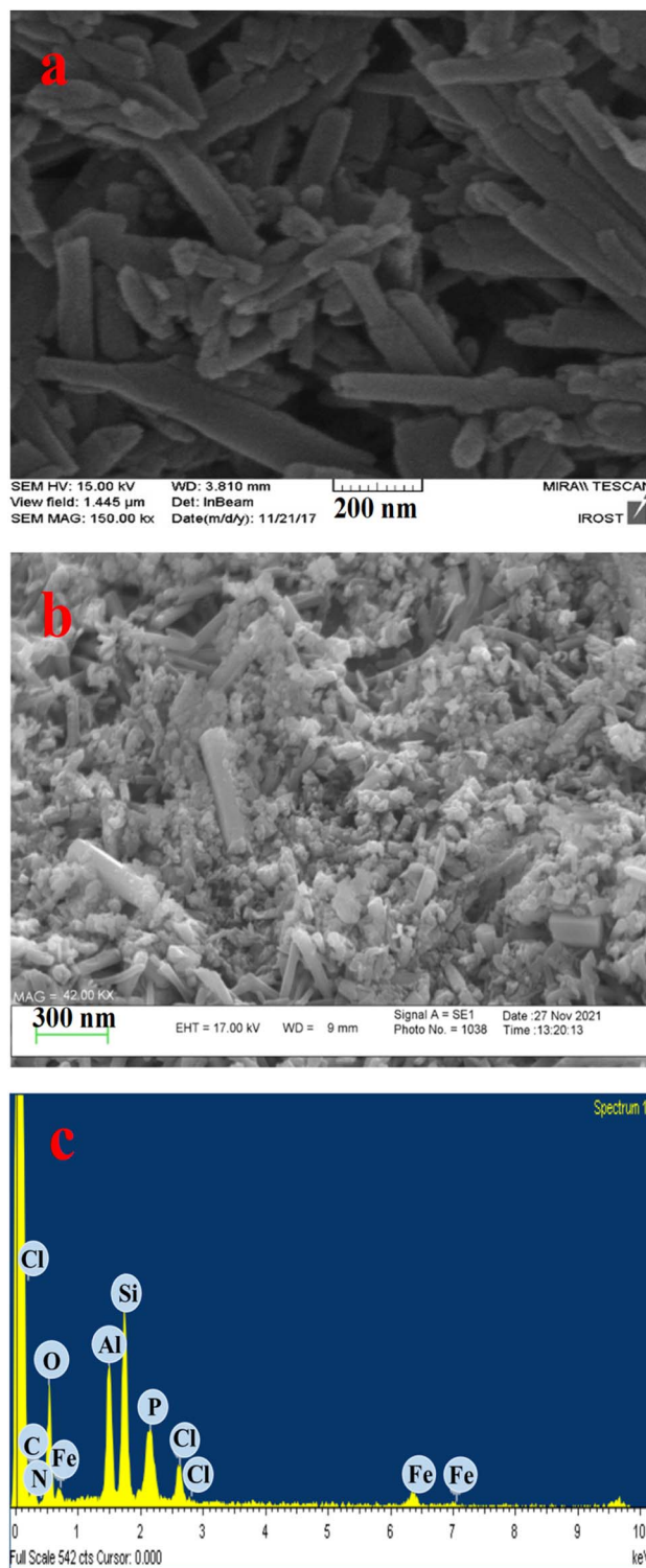
Fig. 3 SEM images of: (a) HNTs, (b) [(APTDP)(FeCl 4 ) 2 @HNT], and (c) SEM/EDX spectrum of [(APTDP)(FeCl 4 ) 2 @HNT].
