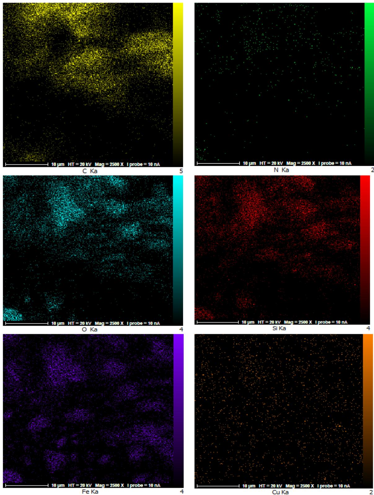
Fig. 5 Corresponding elemental mapping of as-prepared nanocatalyst.
