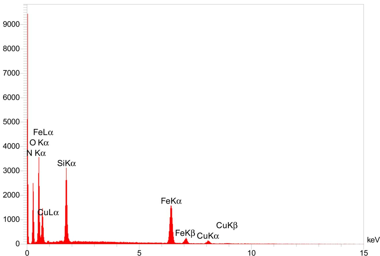
Fig. 4 The EDX spectrum of the Cu(II)-Schiff-base-(CH<sub>2</sub>)<sub>3</sub>@SiO<sub>2</sub>@Fe<sub>3</sub>O<sub>4</sub>.
