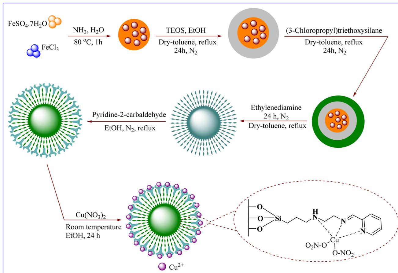
Scheme 2 Synthetic route of magnetic Cu(II)-Schiff-base-(CH<sub>2</sub>)<sub>3</sub>@SiO<sub>2</sub>@Fe<sub>3</sub>O<sub>4</sub>
