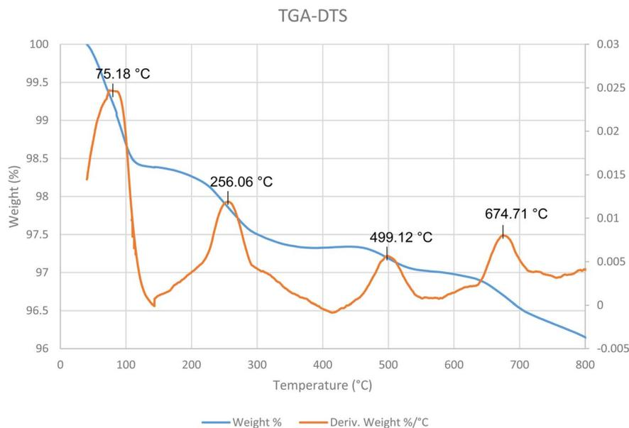
Fig. 6 The TGA-DTS analysis of the as-prepared nanocatalyst.
