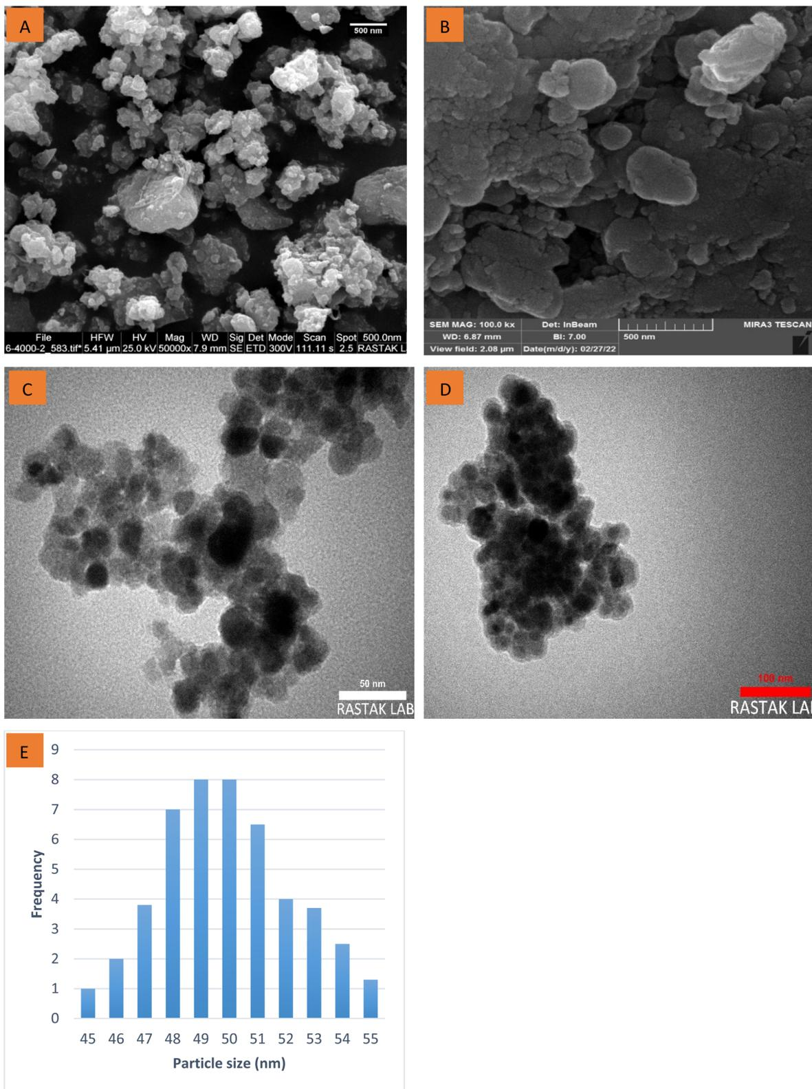
Fig. 3 FE-SEM images of the (A)  $\text{Fe}_3\text{O}_4$  and (B) as-prepared nanocatalyst, TEM images of the (C)  $\text{Fe}_3\text{O}_4$  and (D) as-prepared nanocatalyst, (E) particle size distribution diagram of as-prepared nanocatalyst.
