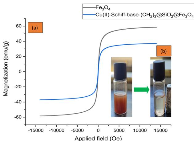
Fig. 8 The VSM analysis of the (a) Fe<sub>3</sub>O<sub>4</sub> and (b) Cu(II)-Schiff-base-(CH<sub>2</sub>)<sub>3</sub>@SiO<sub>2</sub>@Fe<sub>3</sub>O<sub>4</sub> nanocatalyst.
