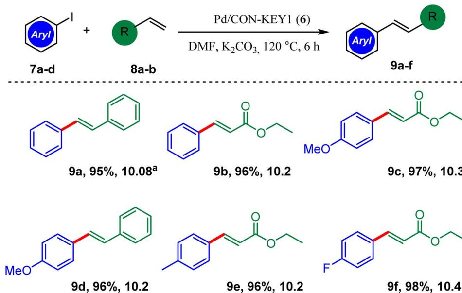
Scheme 3 Heck cross-coupling reactions of aryl iodide with acrylate derivatives and styrene. <sup>a</sup>TON = yield/amount of catalyst (mol).
