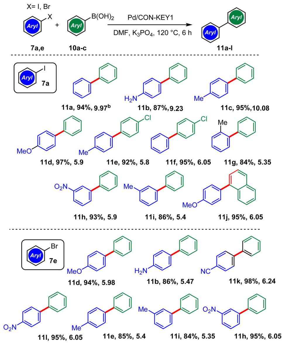
**Scheme 4** Pd/CON-KEY1 catalyzed Suzuki–Miyaura coupling reaction.<sup>a</sup> <sup>a</sup>Reaction conditions: Ar-X **7** (0.5 mmol), ArB(OH)<sub>2</sub> **10** (0.6 mmol), K<sub>3</sub>PO<sub>4</sub> (0.6 mmol) and Pd/CON-KEY1 **6** catalyst (30 mg). <sup>b</sup>TON = yield/amount of catalyst (mol).
