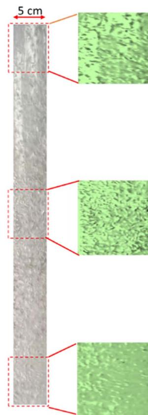
Fig. 2 The bubble formation in the bubble column at different heights using 1% v sodium silicate solution and 2.55 cm s<sup>-1</sup>.
