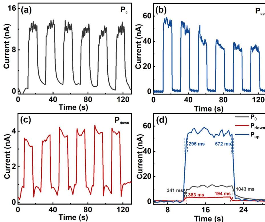
Fig. 4 Photoresponse comparison of InSe/CCPS bilayer device under 300 nm light chopping in (a)  $P_0$ , (b)  $P_{up}$ , and (c)  $P_{down}$  state (d) Comparison of photoresponse time measurement for different polarization states ( $V_{ds}$  of 3 V).
