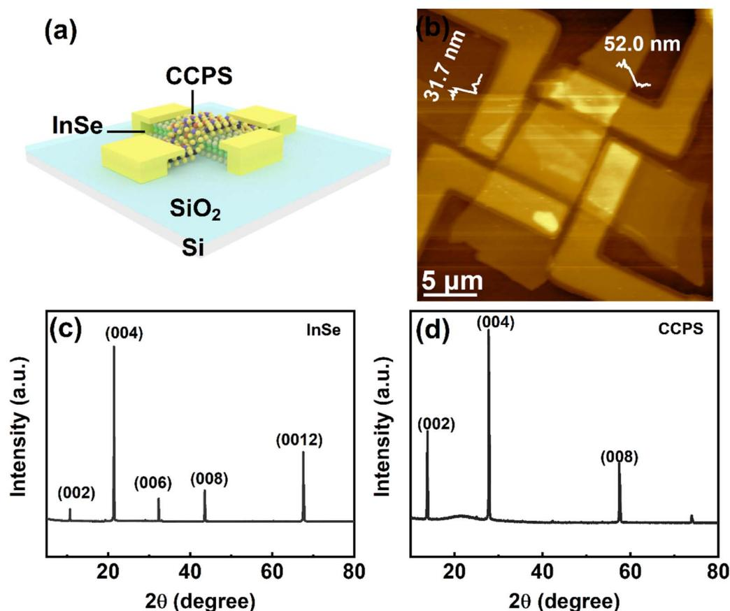
Fig. 1 (a) Schematic illustration of InSe/CCPS device. (b) AFM topography of InSe/CCPS device. XRD spectra of (c) InSe and (d) CCPS.
