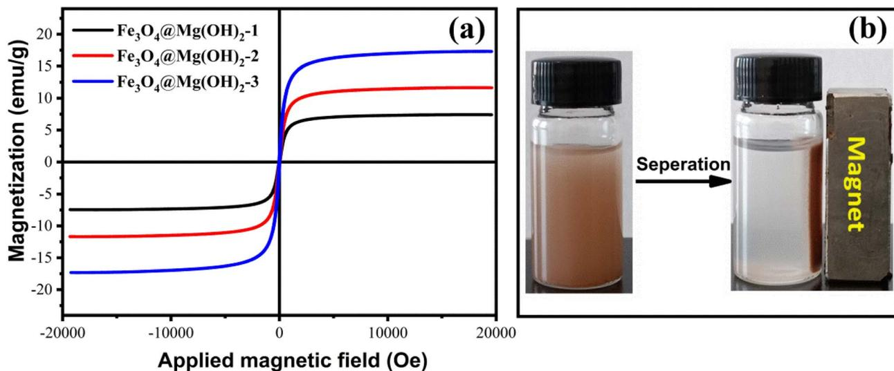
Fig. 1 (a) Magnetic hysteresis loops of  $\text{Fe}_3\text{O}_4@\text{Mg}(\text{OH})_2$  composites obtained at room temperature, (b) magnetic separation process of  $\text{Fe}_3\text{O}_4@\text{Mg}(\text{OH})_2$ -3 composite.
