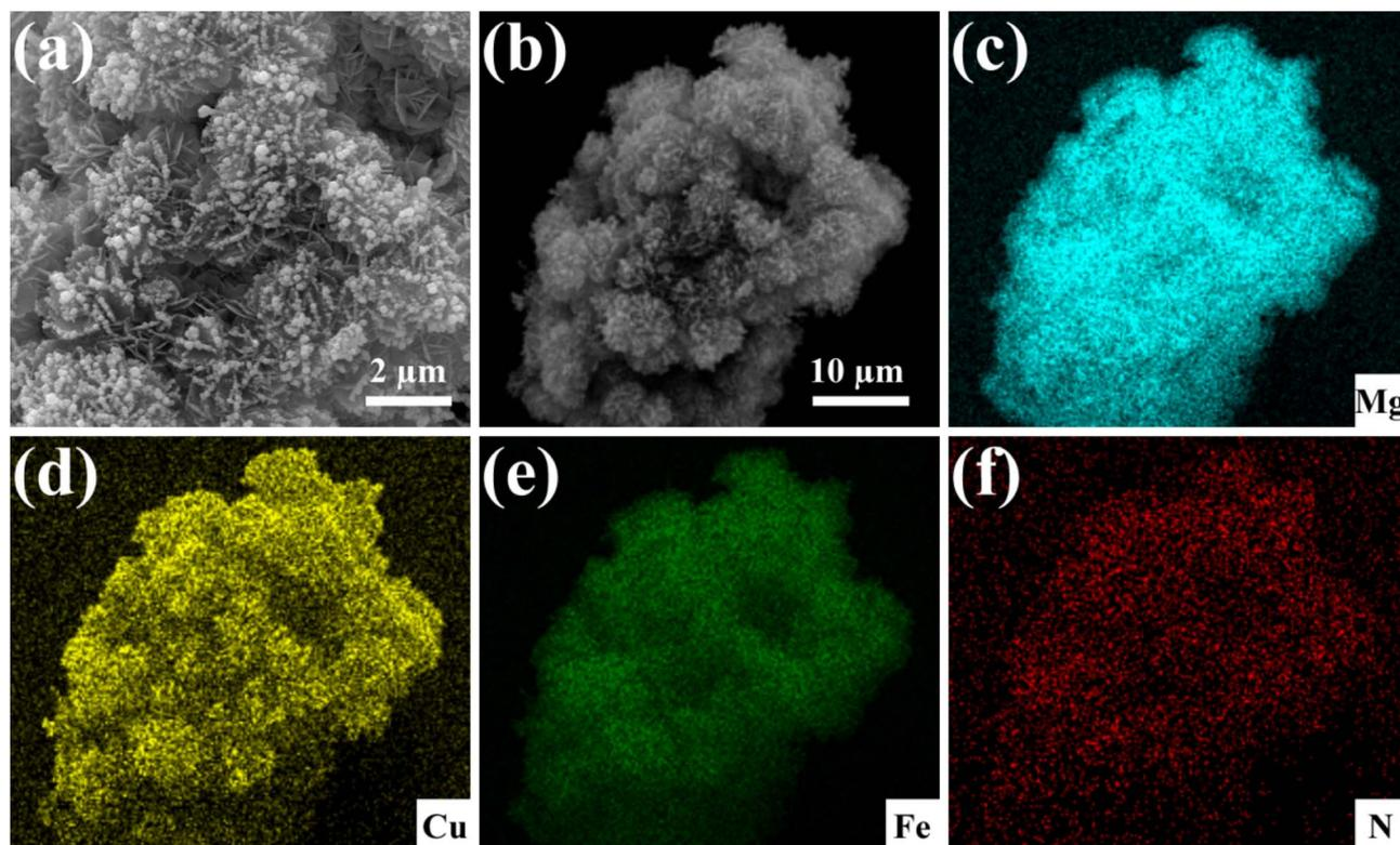
Fig. 9 SEM image of the Fe<sub>3</sub>O<sub>4</sub>@Mg(OH)<sub>2</sub> composites after adsorbing Cu(II) for 10 min (a), along with the corresponding elemental mapping of a selected area (b–f).
