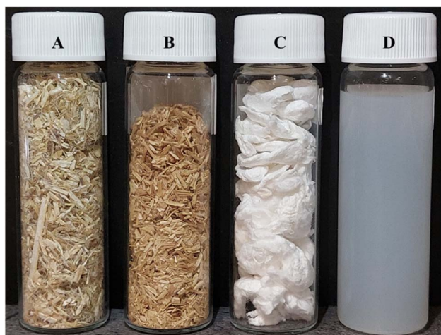
Fig. 2 Photograph of (A) RH, (B) AH, (C) BH and (D) acid hydrolyzed suspension Hemp fibers.
