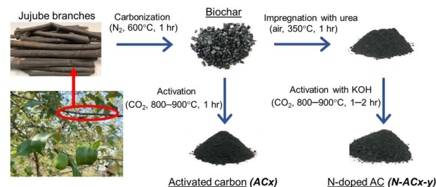
Fig. 1 Synthesis of the original and modified ACs.
