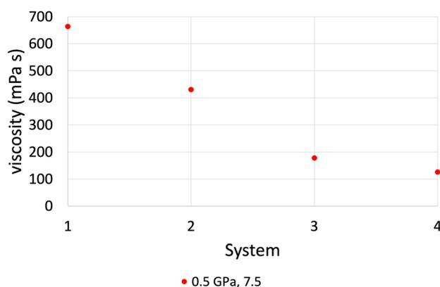
Fig. 6 Viscosity results comparison between confined NEMD simulations (system 1, 2 and 3) and bulk NEMD simulations (system 4) at  $P = 0.5 \text{ GPa}$  and  $\log(\dot{\gamma} [\text{s}^{-1}]) = 7.5$ , by using the L-OPLS-AA force field. As we increase the number of confined lubricant molecules we approach bulk behaviour of viscosity. Systems 1, 2 and 3 contain 100, 200 and 450 lubricant molecules, respectively.
