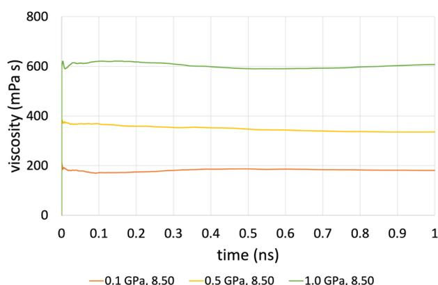
**Fig. 5** Average viscosity of system 2 (200 lubricant molecules), with ReaxFF at a pressure range from 0.1 to 1.0 GPa at 100 °C and at a shear rate of  $10^{8.5} \text{ s}^{-1}$ .
