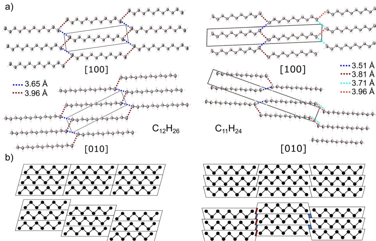
Fig. 2 (a) Crystal structure of *n*-dodecane (left) and *n*-undecane (right) viewed along the crystallographic *a* (top) and *b* (bottom) axes. Thermal ellipsoids are plotted at 50% probability. The shortest intermolecular C–C contacts are underlined with dashed lines; (b) schematic representation of the shift between the layers ([100] view) in even- (left) and odd-numbered (right) alkanes. Red and blue areas indicate shortening and elongation of the intermolecular distances, respectively.
