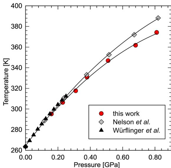
Fig. 4 Phase diagram of *n*-dodecane redetermined in this work (red circles), compared with the densitometric literature data.<sup>76,80</sup>
