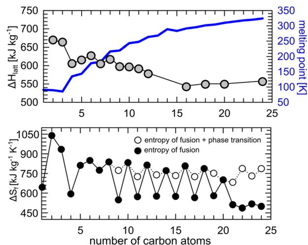
Fig. 3 Top: calculated lattice energies for the crystal structures of  $n$ -alkanes deposited in CSD. Bottom: reported entropies of fusion for  $n$ -alkanes (black circles) and entropies of fusion corrected by the addition of the entropy change between crystalline and premelting rotator phases (white circles).
