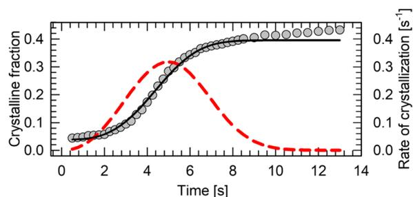
**Fig. 7** Crystallization kinetics of dodecane at 0.15(3) GPa. The crystalline fraction is a ratio between the measured surfaces of the crystal and the DAC chamber (grey circles), fitted with Avrami model (black curve). The first derivative of the model with respect to time (crystallization rate) is depicted as a red curve.
